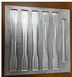
FIG. A1. Tensile mold made of aluminum.
