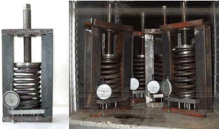
FIG. 1. View of the device used to determine creep curves with mounted and loaded specimens.
