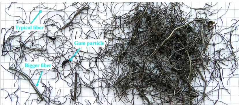
**FIG. 1.** Fibers from end-of-life tires – recycled steel fibers (RSF).
