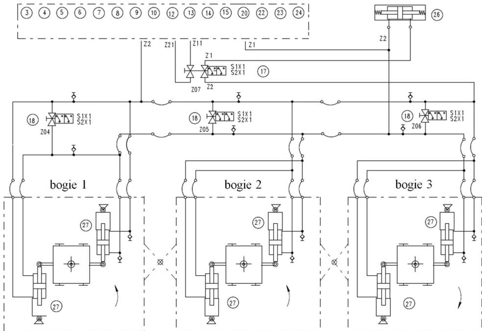
FIG. 4. Hydraulic outline of the system (description in the text).
