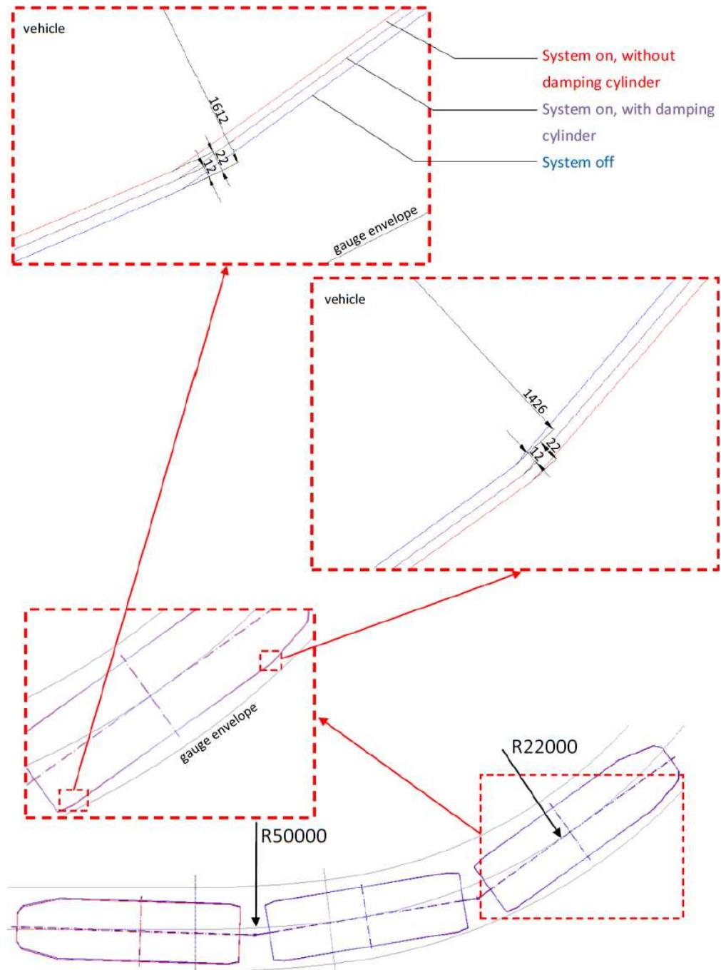
FIG. 8. Kinematic gauge compatibility check for various system states
