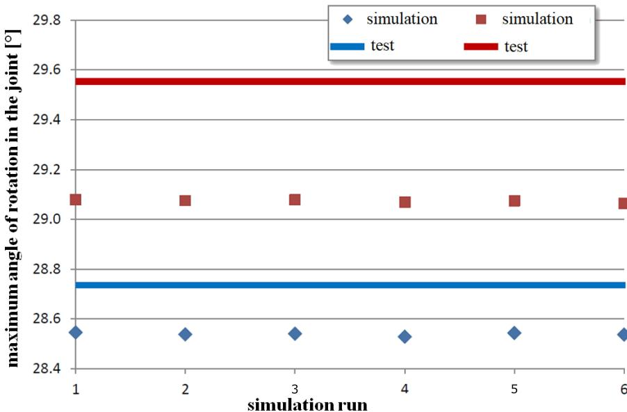
FIG. 11. Angle of rotation between cars – reduced equivalent stiffness of the system (100 kN/mm).
