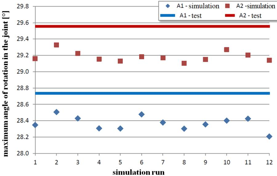
FIG. 12. Angle of rotation between cars – reduced equivalent stiffness of the system (0.48 kN/mm).
