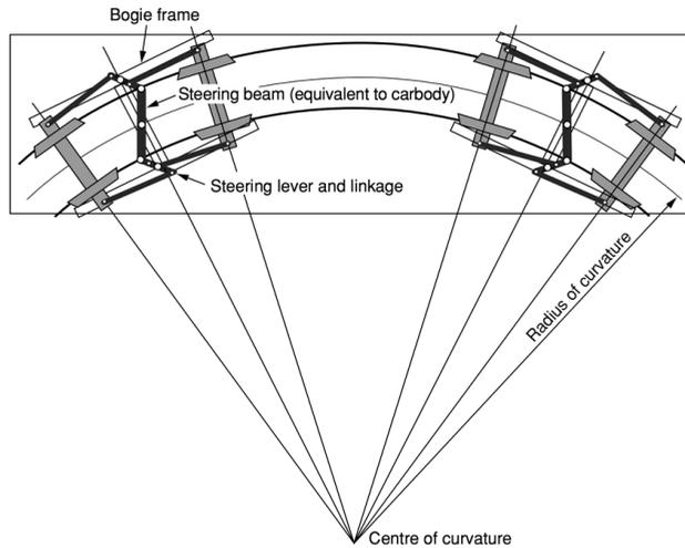
FIG. 1. Radial steered wheelsets [1].
