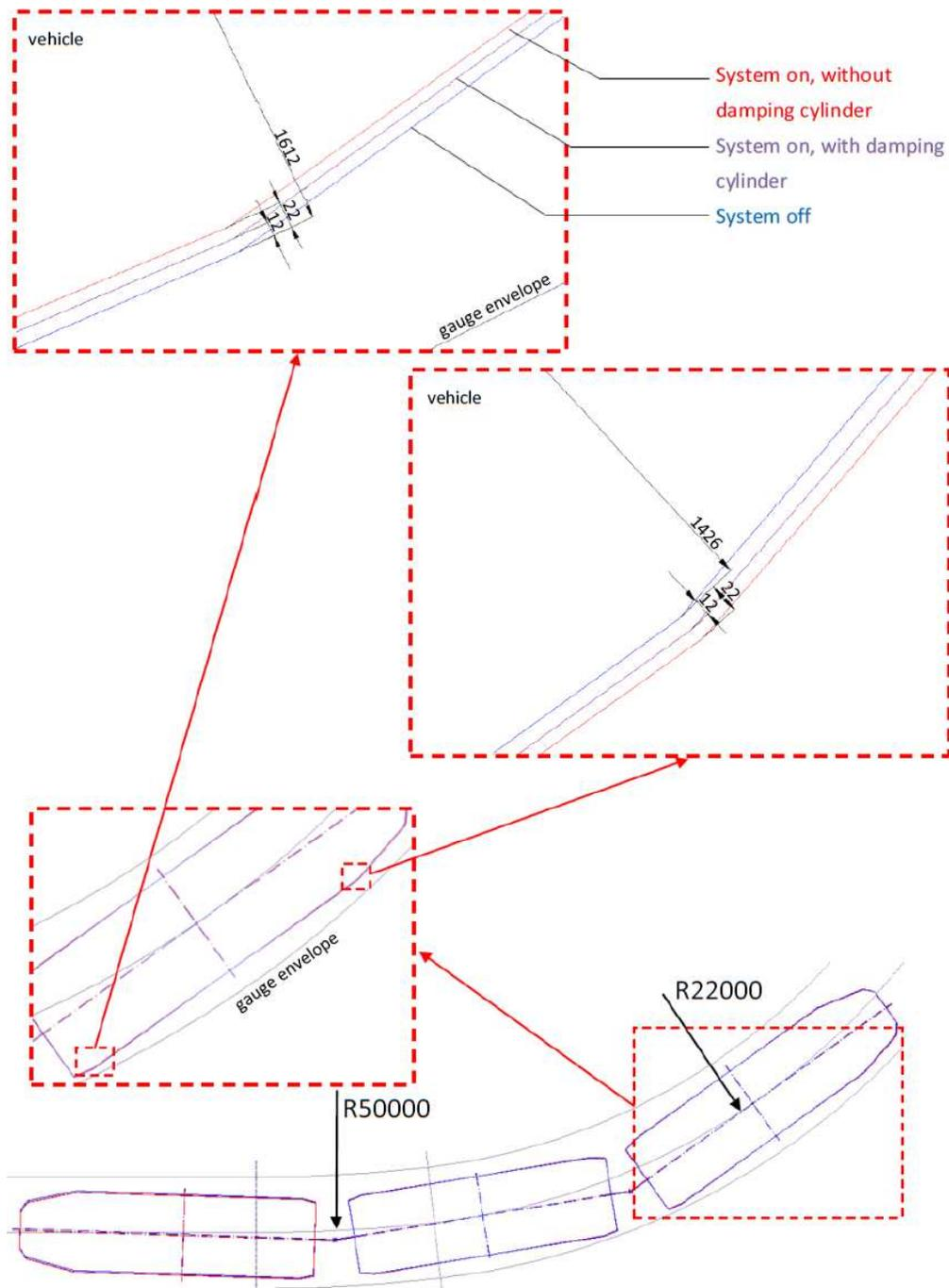
FIG. 8. Kinematic gauge compatibility check for various system states (in mm, description in text).
