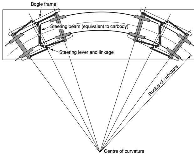
FIG. 1. Radial steered wheelsets [1].
