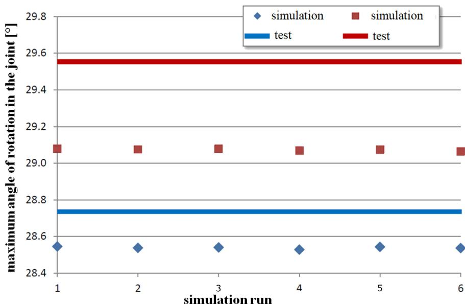
FIG. 11. Angle of rotation between cars – reduced equivalent stiffness of the system (100 kN/mm).
