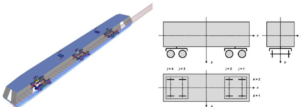
FIG. 10. Vehicle model view and coordinate system adopted for simulation [15].
