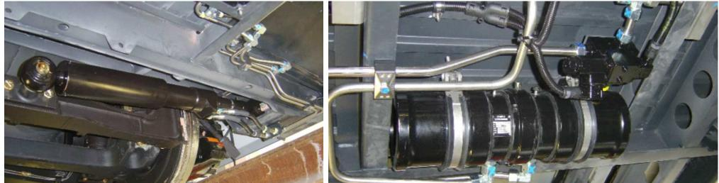
FIG. 3. Left: hydraulic damper connecting bogie and carbody, right: hydraulic damper's cylinder [3].
