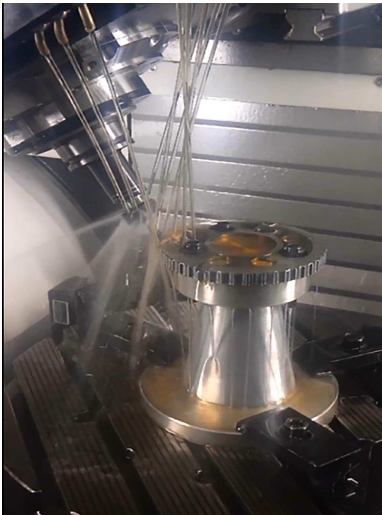
FIG. 2. Process of five-axis end milling of cycloidal gears.
