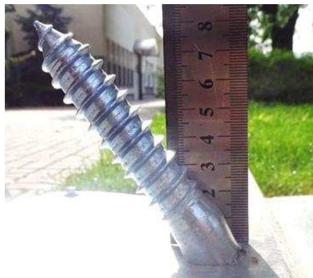
FIG. 7. The failure mode in the connector.
