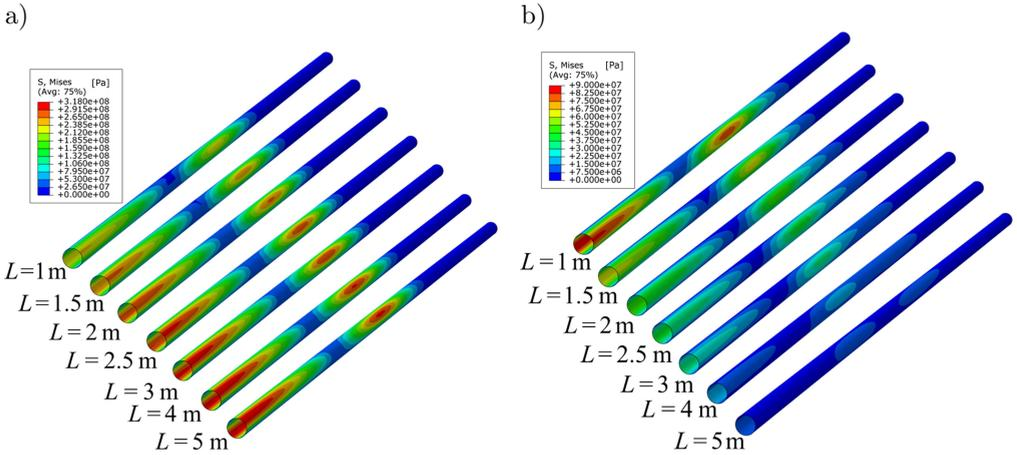
FIG. 2. Stress of the pipeline under different parallel distances: a) pipeline-1, b) pipeline-2.
