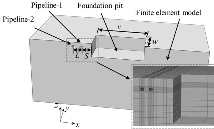
FIG. 1. Schematic diagram of foundation pit.
