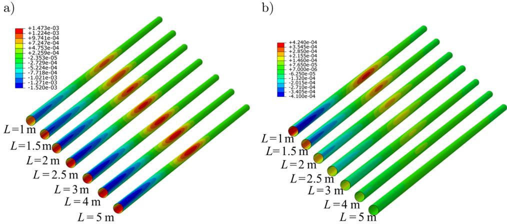
FIG. 4. Axial strain of the pipeline under different parallel distances: a) pipeline-1, b) pipeline-2.
