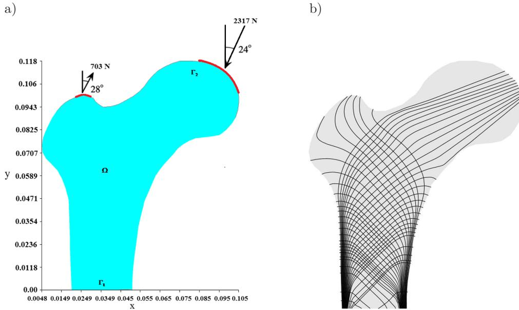
FIG. 1. a) Setting of the static problem, b) trajectories of principal stresses in the optimal body.
