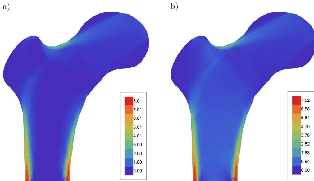
FIG. 2. Optimal layouts of: a) elastic modulus  $a/(100E_0)$ , b) elastic modulus  $c/(100E_0)$ .
