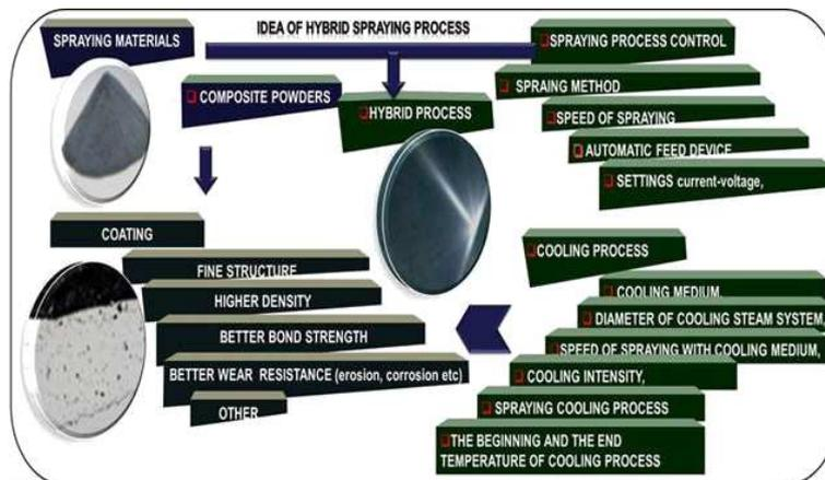
FIG. 3. Idea of hybrid spraying process.
