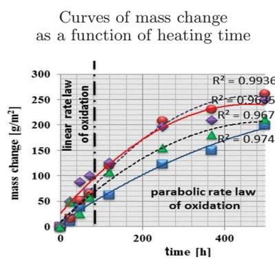
The analysis of curves leads to the conclusion that for each tested coating, after an initial period of rapid weight growth, the stabilization period of oxidation is registered. This period is compatible with the parabolic rate law of oxidation.
