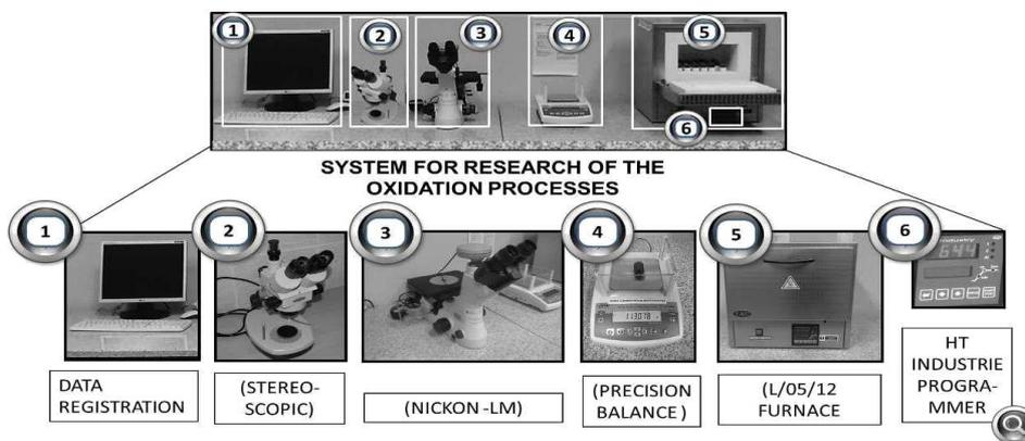
FIG. 4. Research corrosion stand.
