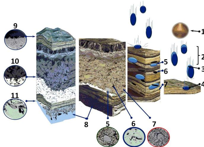
FIG. 1. Building a full coating of a desired thickness: 1 – heat source (arc, flame), 2 – speeding up particles, 3 – oxide coating, 4 – blowing particles into the ground, 5 – non-molten particles, 6 – pores, 7 – oxide layers, 8 – base material, 9 – surface roughness, 10 – transition zone in the coating layered, 11 – transition zone between the coating.
