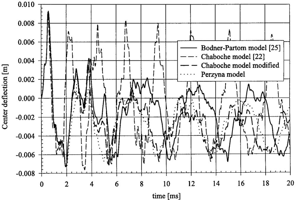
FIG. 7. Dynamic response of INCO718 plate at  $650^{\circ}\text{C}$  to explosive type of loading.
