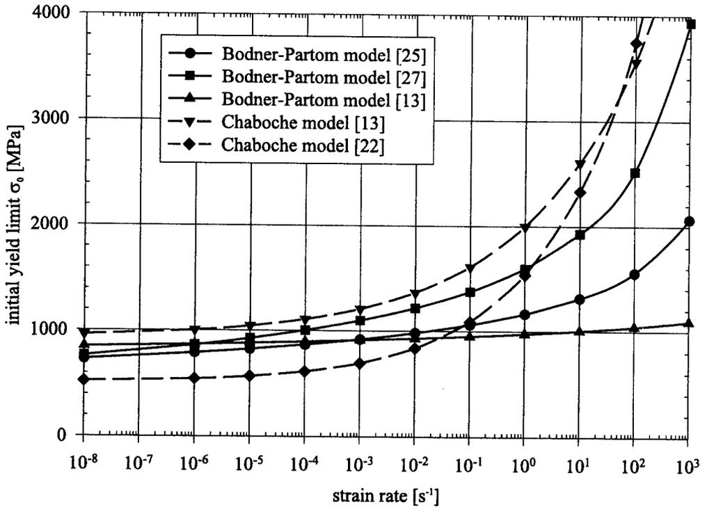
FIG. 1. Initial yield limit as the function of strain rate for INCO718 at 650° C.
