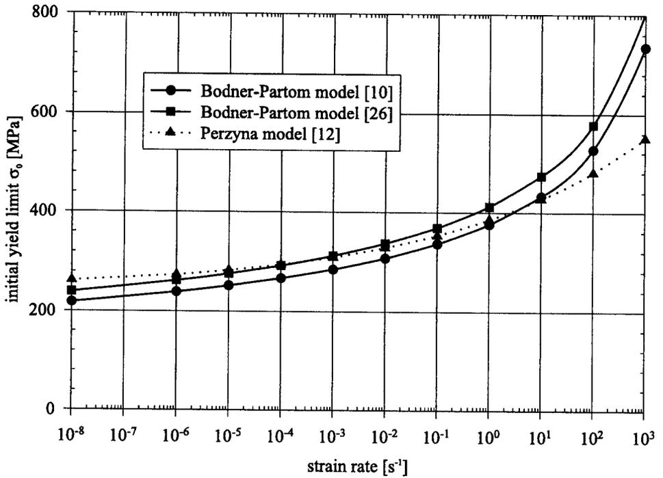
FIG. 3. Initial yield limit as the function of strain rate for titanium at 20° C.
