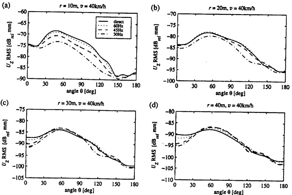
FIG. 2. RMS vertical soil displacements due to a train speed of 40 km/h at radii of (a) 10 m; (b) 20 m; (c) 30 m and (d) 40 m from the tunnel centre-line. The variation with angular position around the tunnel is given -  $\theta = 0$  corresponding to vertically downwards - and the effect of different slab bearing stiffnesses is shown, including direct coupling to the tunnel.
