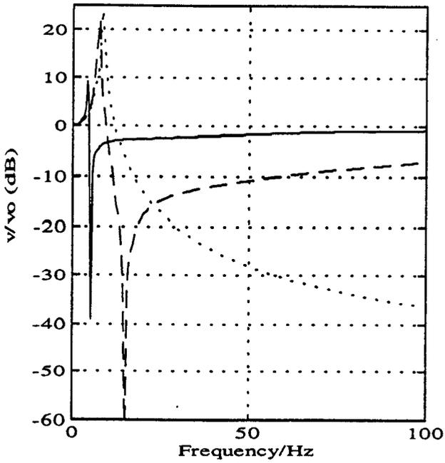
FIG. 6. The effect of a SDOF model on the ground vibration-field; (solid) 5 Hz (dashed) 15 Hz and (dotted) 'infinitely stiff' isolation.
