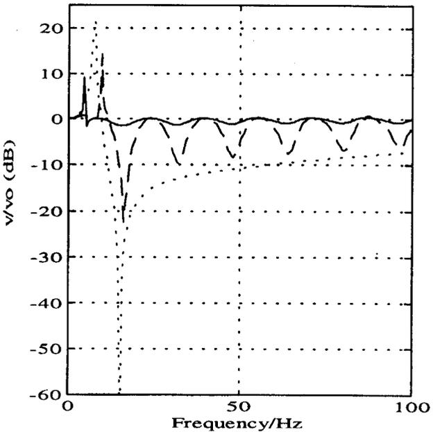
FIG. 7. The effect of a 2-DOF model on the ground vibration-field; (solid) 5 Hz and (dashed) 15 Hz isolation. 15 Hz SDOF case also shown (dotted).
