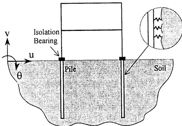
FIG. 3. Model of a base-isolated building. The building is represented by a two-dimensional portal frame while the piled foundation is based on a three-dimensional representation due to Gazetas and Makris. The pile-soil interface is represented by distributed springs and dashpots. For clarity, only the horizontal springs are shown.
