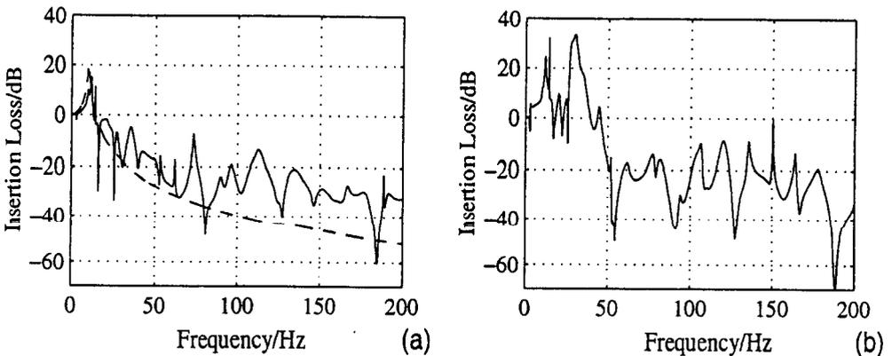
FIG. 4. Variation with frequency in the (a) vertical and (b) horizontal insertion loss of a '10 Hz' base-isolated building. The response of a rigid-body SDOF model is shown dashed for comparison.
