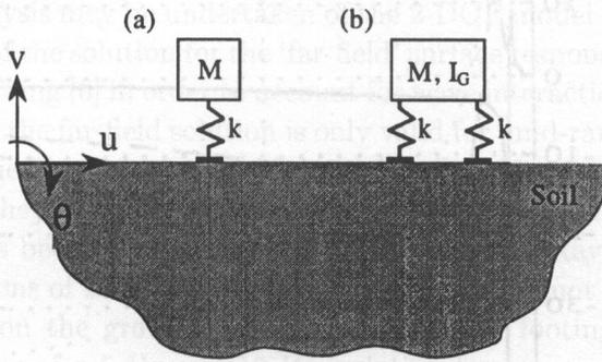
FIG. 5. Rigid-body models of a base-isolated building founded on an elastic half-space.
