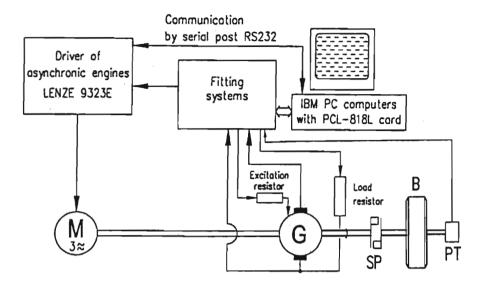
Fig. 3. Block diagram of the test stand M – alternative current machine, G – direct-current generator, SP – clutch, B – inertia mass, PT – tachometer generator.
