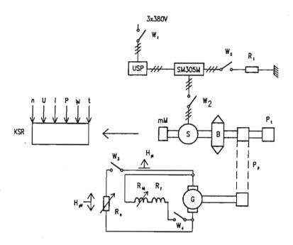
Fig. 2. Schematic diagram with direct-current generator (medium voltage) USP – control and measuring system, SM305M – controller, R<sub>1</sub> – additional load resistor (brake),
