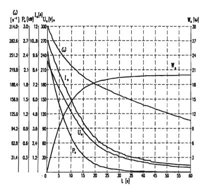
Fig. 12. Current, voltage, power angular speed and recovered energy versus time for shunt direct-current generator during braking the inertia mass from the angular speed of 314 s<sup>-1</sup>.
