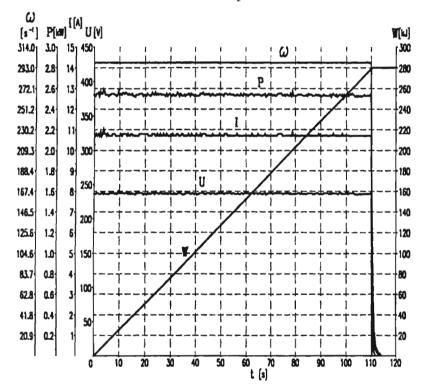
Fig. 11. Current, voltage, power, angular speed and recovered energy versus time graphs for shunt direct-current generator during loaded sheave block lowering phase  $(\omega = 298.3 \text{ s}^{-1}, P = 2.5 \text{ kW}).$
