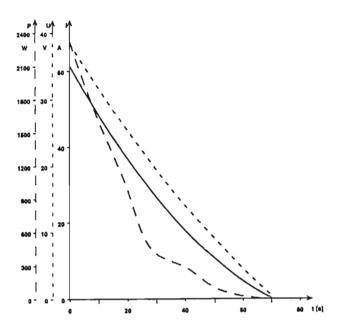
Fig. 7. Current, voltage and power versus time graphs for direct-current generator during braking phase with energy transmission to the load resistor ( $\omega = 293 \text{ s}^{-1}$ ,  $R = 0.23 \Omega$ ).
