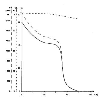
Fig. 8. Current, voltage and power versus time graphs during braking phase with energy transmission to the electrochemical battery ( $\omega = 293 \text{ s}^{-1}, 34 \text{ Ah}$ ).
