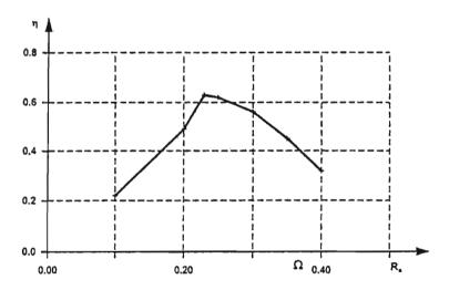
Fig. 6. Efficiency of energy recovery versus load resistance ( $\omega = 293 \text{ s}^{-1}$ ).
