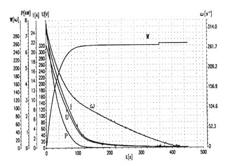
Fig. 10. Current, voltage, power, angular speed, recovered energy versus time graphs for a shunt direct-current generator during braking the inertia mass from the angular speed of 314 s<sup>-1</sup>.
