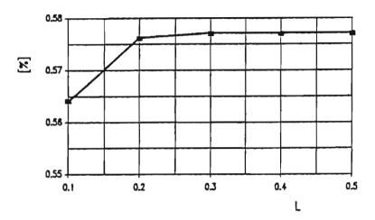
Fig. 5. Efficiency of energy recovery versus discharge factor of 34 Ah battery for angular speed change from 293 s<sup>-1</sup>.
