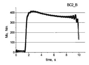
Fig. 9. Braking torque for the BC2\_B drum.
