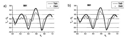
Fig. 5. Temperature and a roundness deviation of the BB1 drum in the section passing through points A and B.
