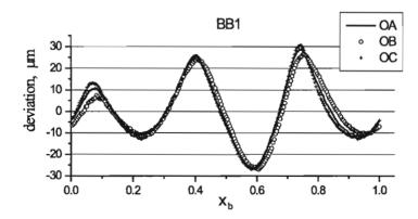
Fig. 4. Roundness deviations for the BB1 drum in sections A, B and C (see Fig. 2a).
