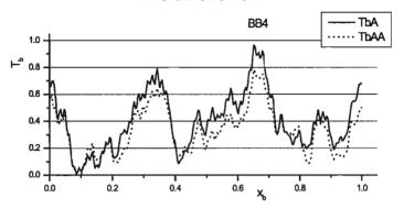
Fig. 8. Distribution of temperature on the outer surface of the BB4 drum from the side of the concurrent  $(T_bA)$  and backward  $(T_bAA)$  shoe.
