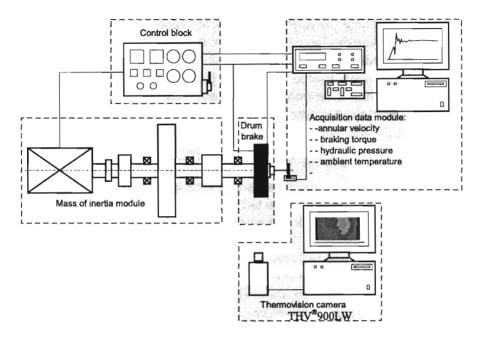
Fig. 1. Block diagram of the stand for testing brakes.
