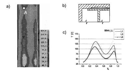
Fig. 6. Concurrent shoe of the BB4 drum: a) thermograph of the surface, b) diagram of the contact of the drum and the shoe, c) distribution of temperature along the generating line of the drum.
