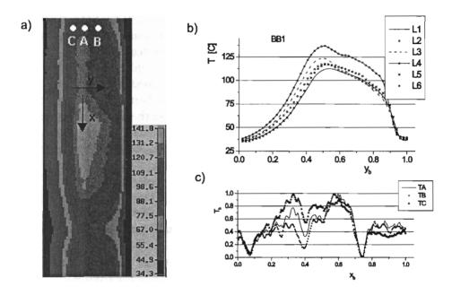
FIG. 2. The BB1 drum (the 21-st revolution): a) thermograph of a segment of the outer surface of the drum, b) distribution of temperatures along the generating line of the drum, along  $y_b$ , c) distribution of temperature on the circumference of the drum, along  $x_b$  for points A, B and C.
