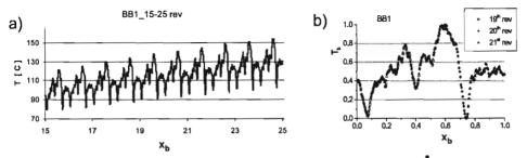
Fig. 3. Temperature on the circumference of the BB1 drum at point A: a) for ten consecutive revolutions (from the 16<sup>th</sup> to 25<sup>th</sup>), b) for three consecutive revolutions (19<sup>th</sup>, 20<sup>th</sup> and 21<sup>st</sup>).
