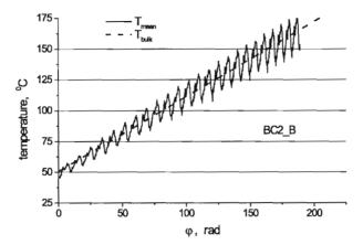
Fig. 11. Mean and bulk drum temperature changes in the BC2 B braking process.
