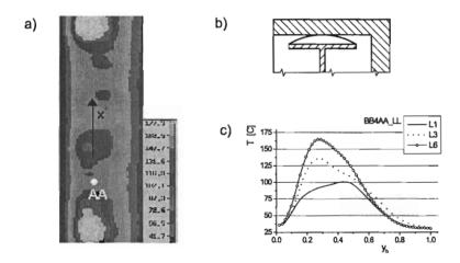
Fig. 7. Backward shoe of the BB4 drum: a) thermograph of the surface, b) diagram of the contact between the drum and the shoe, c) distribution of temperature along the generating line.
