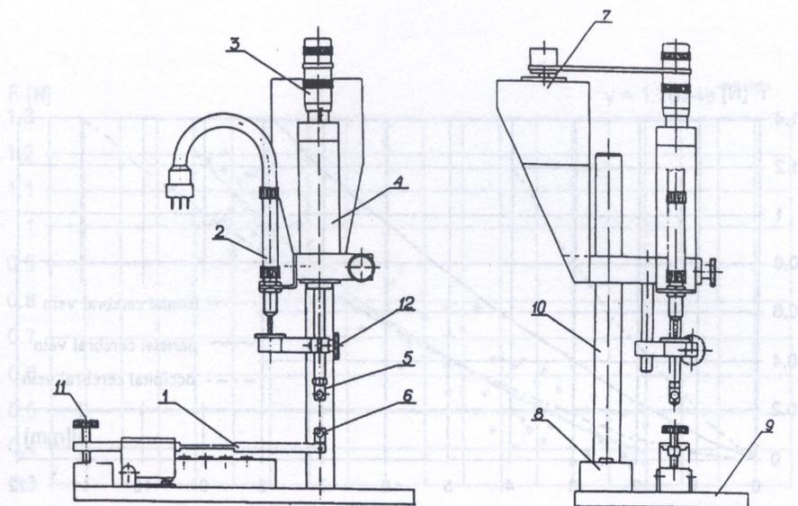
FIG. 2. Microscarifier: 1 - force gauge beam, 2 - linear extension sensor, 3 - analog displacement indicator, 4 - tightener unit, 5 - upper mount seat, 6 - lower mount seat, 7 - actuator, 8 - force gauge electrical unit, 9 - base of microscarifier, 10 - column, 11 - preliminary tension correction screw, 12 - preliminary tension control knob.
