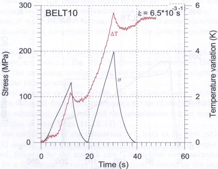
FIG. 13. Stress and temperature vs. time of woven polyamide belt subjected to two subsequent cycles of loading and unloading.
