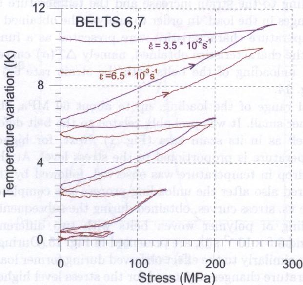
FIG. 15. Temperature changes vs. stress obtained for woven polymer belt during subsequent tension tests with strain rates  $6.5 \times 10^{-3} \text{ s}^{-1}$  and  $3.5 \times 10^{-2} \text{ s}^{-1}$ .
