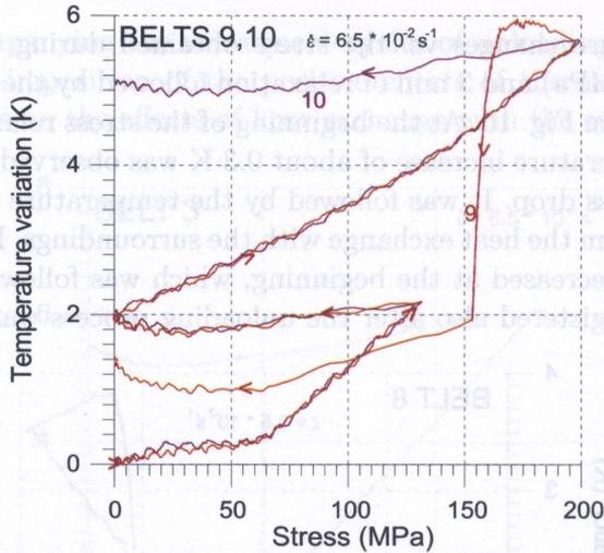
FIG. 17. Comparison of the temperature changes vs. stress obtained for two woven polymer belts subjected to subsequent cycles of loading with relaxation sequences (curve 9) and without relaxation (curve 10).
