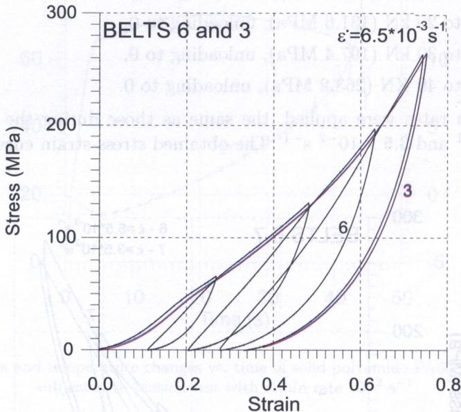
FIG. 8. Comparison of two tests: stress-strain curve (3) and subsequent low-cyclic tests (6), obtained for the polyamide woven belts subjected to tension tests with strain rate  $6.5 \times 10^{-3} \text{ s}^{-1}$ .
