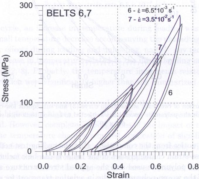
FIG. 7. Stress-strain curves, obtained for the polyamide woven belts subjected to low-cyclic tests with two different strain rates:  $6.5 \times 10^{-3} \text{ s}^{-1}$  and  $3.5 \times 10^{-2} \text{ s}^{-1}$ .
