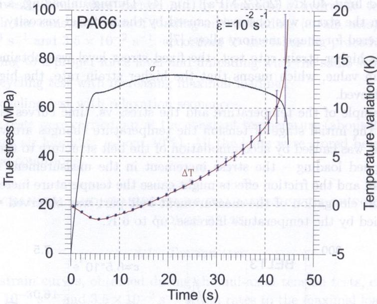
FIG. 6. Stress and temperature changes vs. time of solid polyamide PA66 sheet sample subjected to tension test with strain rate  $10^{-2} \text{ s}^{-1}$ .
