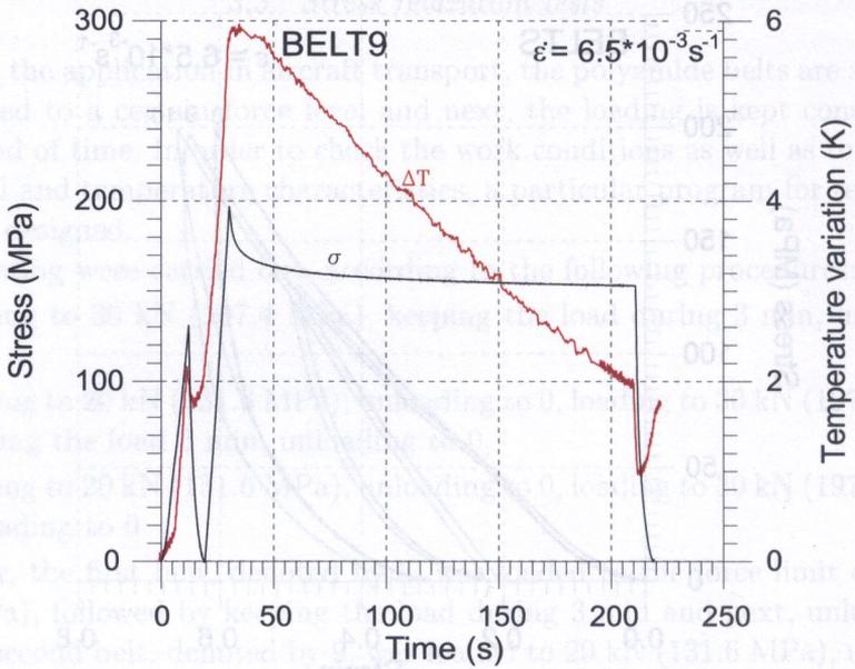
FIG. 12. Stress and temperature vs. time of woven polyamide belt subjected to loading, unloading and stress relaxation sequences in the second cycle of loading.
