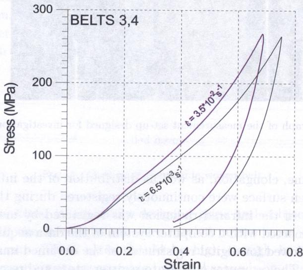
FIG. 4. Stress-strain curves, obtained during uni-axial tension tests of polyamide woven belt for two different strain rates:  $6.5 \times 10^{-3} \text{ s}^{-1}$  and  $3.5 \times 10^{-2} \text{ s}^{-1}$ .
