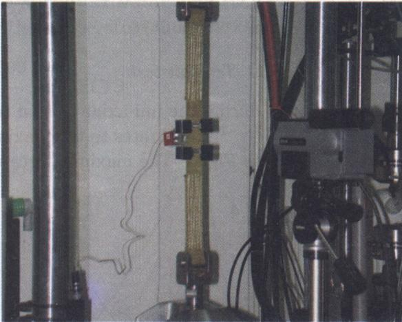
FIG. 3. Photograph of the measurement set-up designed for investigation of polyamide woven belt.
