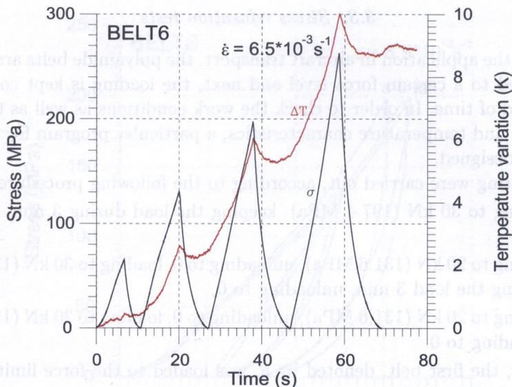
FIG. 9. Stress and temperature curves of polyamide woven belt subjected to subsequent cyclic test with strain rate  $6.5 \times 10^{-3} \text{ s}^{-1}$ .
