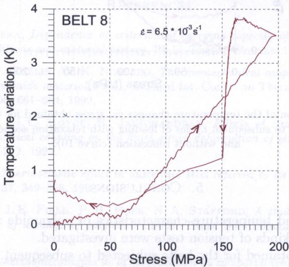
FIG. 16. Temperature changes vs. stress obtained during the relaxation test of woven polymer belt.
