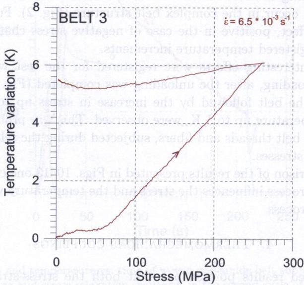
FIG. 14. Temperature changes vs. stress of woven polymer belt subjected to loading and unloading during tension test with the strain rate  $6.5 \times 10^{-3} \text{ s}^{-1}$ .
