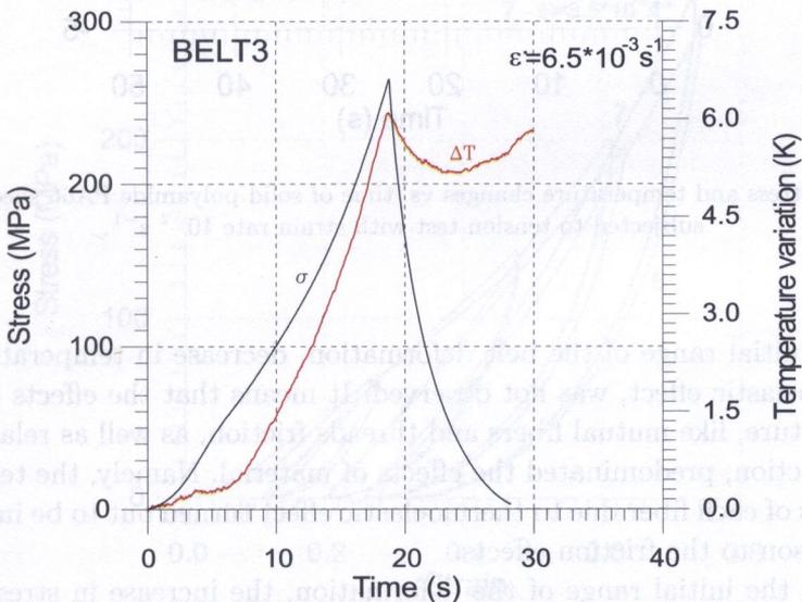
FIG. 5. Stress and temperature changes vs. time of polyamide fiber belt subjected to tension test with strain rate  $6.5 \times 10^{-3} \text{ s}^{-1}$ .
