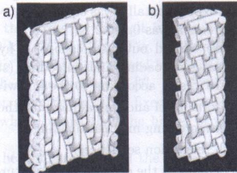
FIG. 2. Macroscopic structure of polyamide woven belt: a) cross-section parallel to the belt surface, b) cross-section perpendicular to the belt surface [6].
