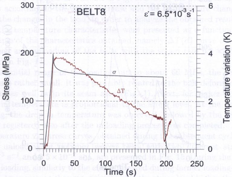
FIG. 11. Stress and temperature vs. time of woven polyamide belt subjected to tension and stress relaxation tests.
