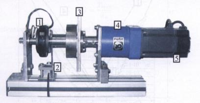
FIG. 12. Experimental setup: 1 – MR brake, 2 – strain gauge, 3 – rigid clutch, 4 – planetary gearbox, 5 – servomotor.
