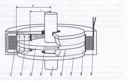
FIG. 2. Diagram of an MR brake.
