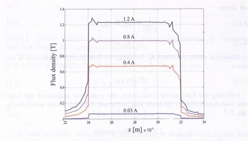
FIG. 8. Flux density distribution along the gap for various current levels.
