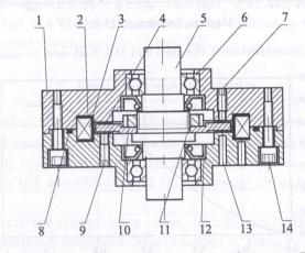
FIG. 6. Brake structure: 1 - housing, 2 - carcass, 3 - coil, 4 - gap, 5 - shaft, 6 - bearing,
