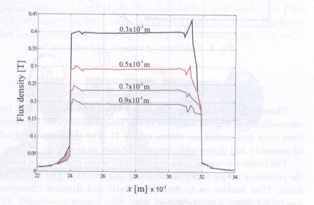
FIG. 7. Flux density distribution along the gap for various gap sizes.
