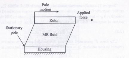
FIG. 1. MR fluid in direct-shear mode.
