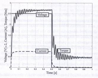
FIG. 15. Current and torque responses to step voltage input for A = 5 V.
