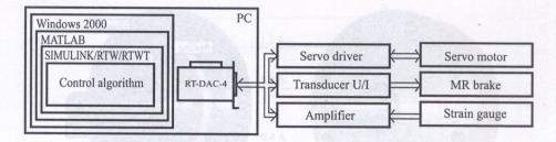
FIG. 13. Block diagram of the experimental setup.
