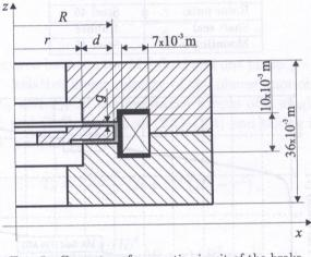
FIG. 5. Geometry of magnetic circuit of the brake.
