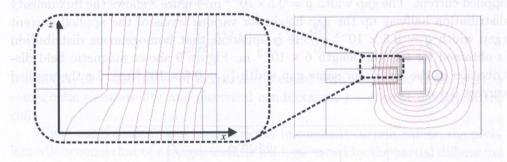
FIG. 9. Distribution of magnetic field within the brake.
