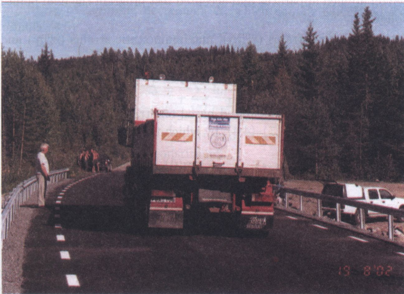
FIG. 3. Passing and braking the Scania vehicle on the bridge with a speed of 60 km/h.
