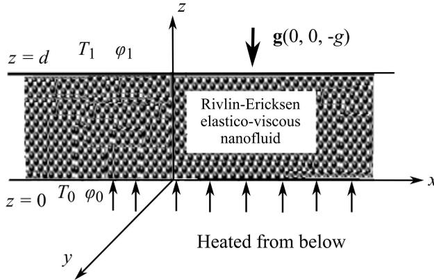
FIG. 1. Schematic sketch of the physical situation.
