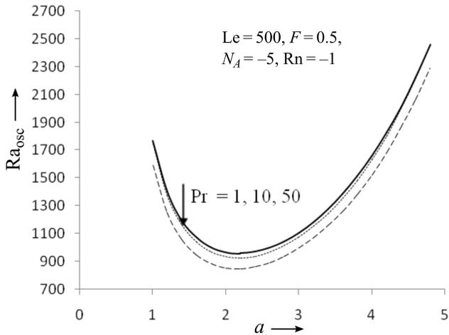
FIG. 7. Variation of oscillatory Rayleigh number with wave number for different Prandtl number.
