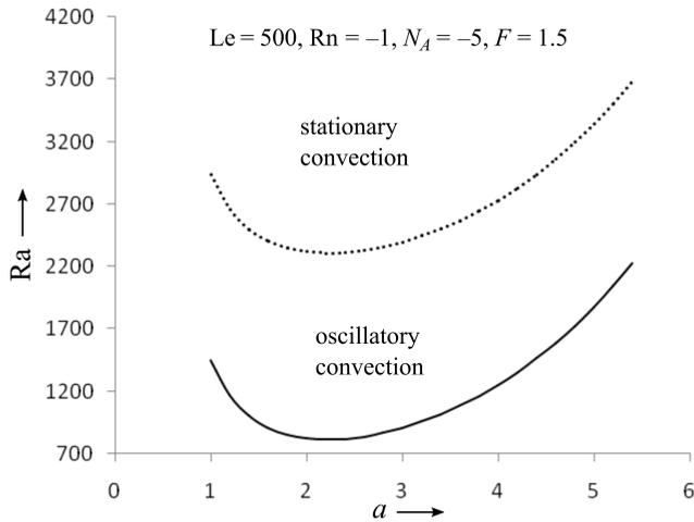
FIG. 10. Variation of stationary Rayleigh number and oscillatory Rayleigh number with wave number.
