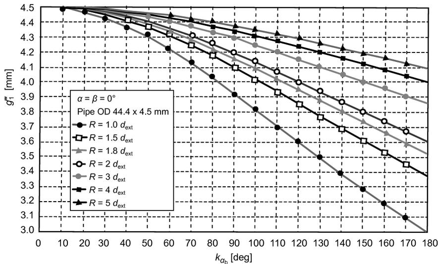
FIG. 4. Wall thickness at the apex point as a function of bending angle for selected values of the bending radius [1].
