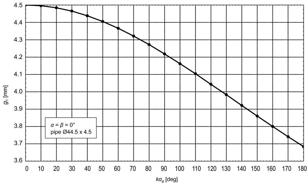
FIG. 7. Variation of the wall thickness at the apex point of the elongated area, where  $\alpha_g \equiv \alpha_b$ .
