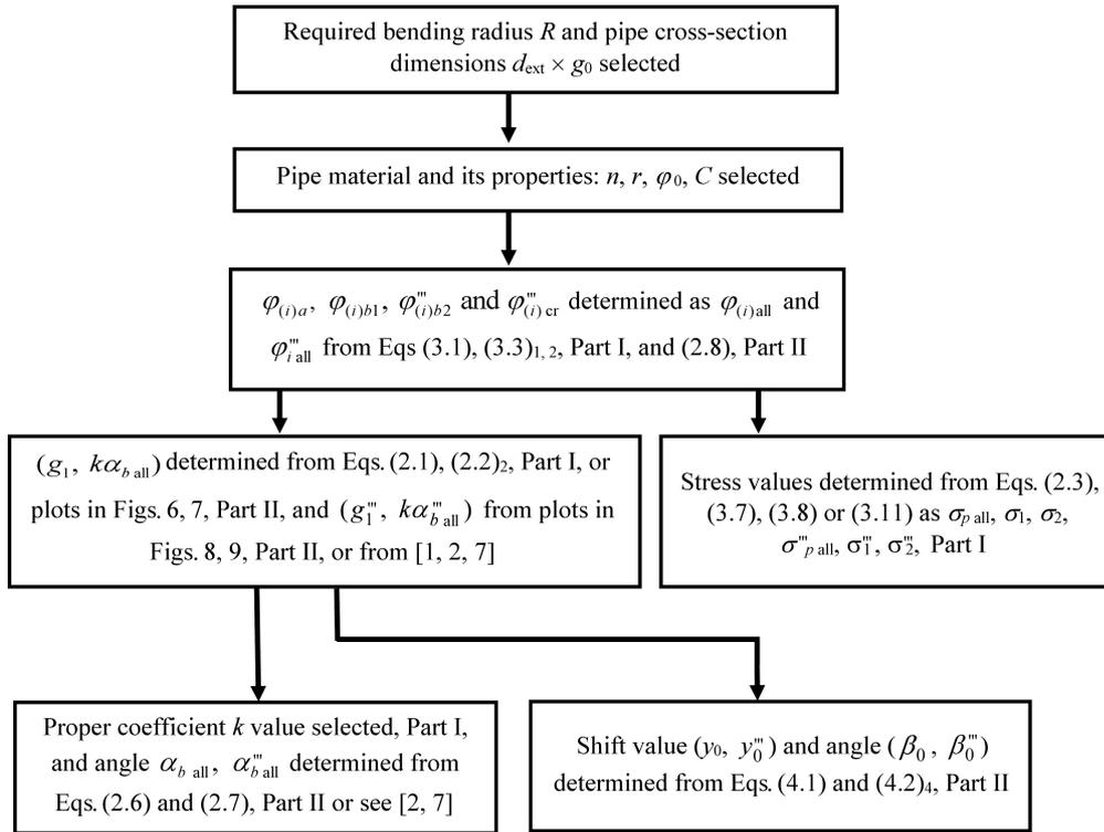
FIG. 10. Flow chart showing the computation stages.
