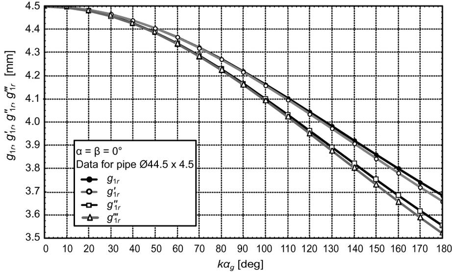
FIG. 8. Variation of the wall thickness value at the bend apex versus bending angle according to four computing methods, where  $\alpha_g \equiv \alpha_b$ .
