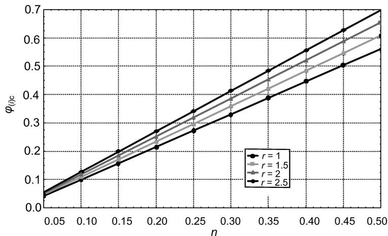
FIG. 2. Admissible equivalent strains as a function of the normal anisotropy index for selected values of the hardening exponent [1].
