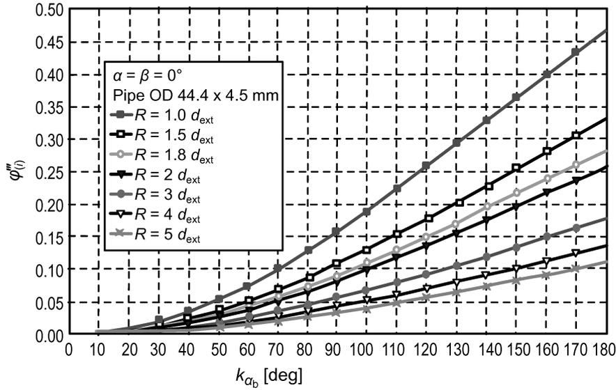
FIG. 5. Equivalent strain value at the bend apex point as a function of bending angle for selected values of the bending radius [1].
