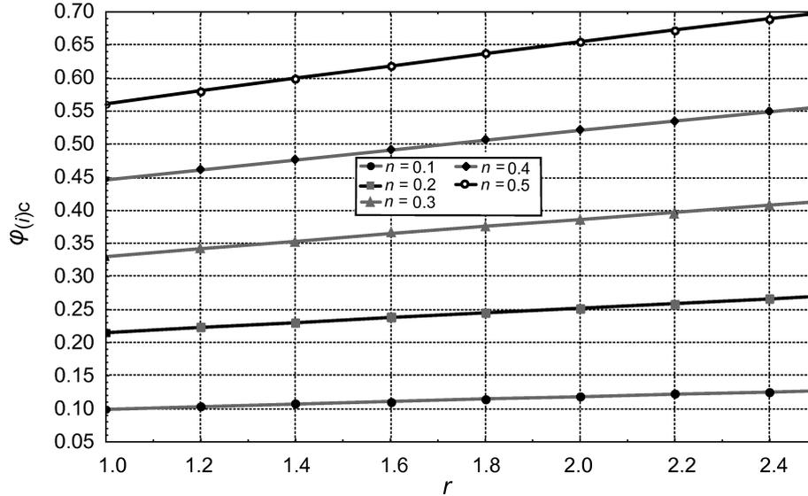
FIG. 3. Admissible equivalent strain as a function of the normal anisotropy index  $r$  for selected values of the hardening exponent [1].
