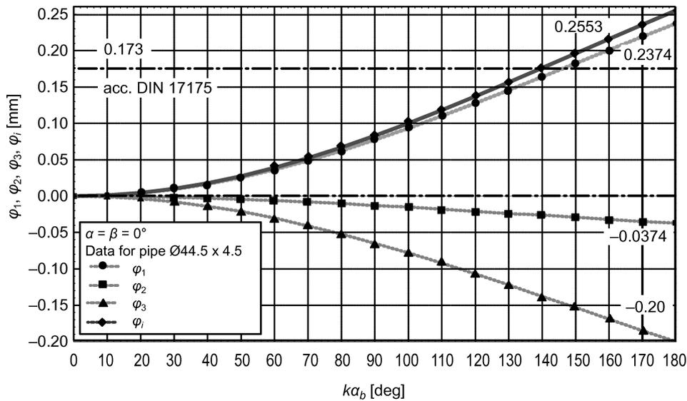
FIG. 6. Strain and strain intensity components as functions of the bending angle, where  $\alpha_g \equiv \alpha_b$ .
