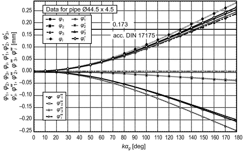
FIG. 9. Strain components and strain intensity versus the bending angle according to three computing methods ( $\alpha_g \equiv \alpha_b$ ).
