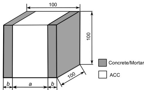
FIG. 1. 3D view of composite block.
