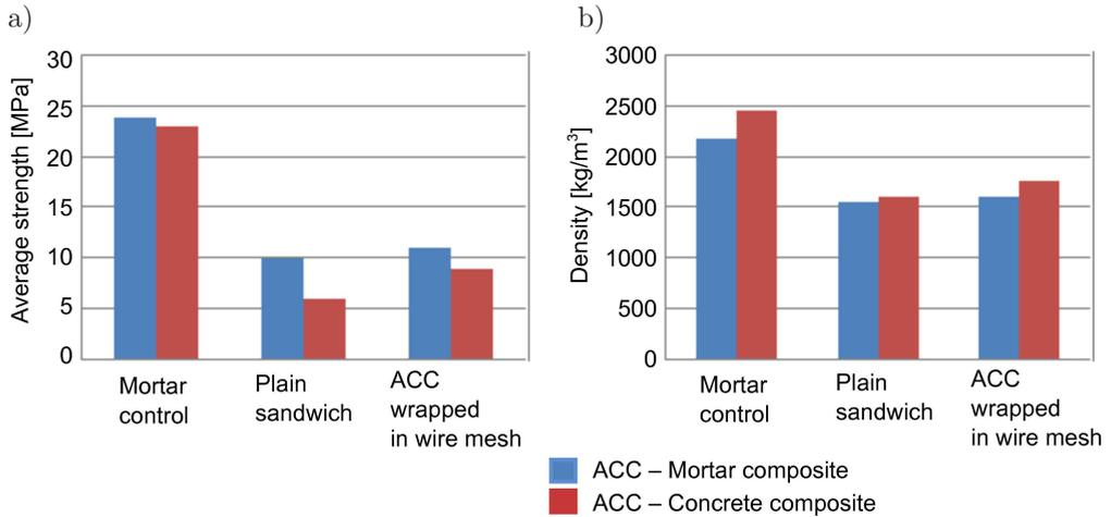
FIG. 5. Test results for the second set of composite block specimens at 3 days using a 3.0 MPa AAC: a) average strength, b) density.
