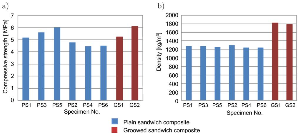
FIG. 9. Compressive strengths and corresponding densities of grooved and plain sandwiches at quasi-static loading rates: a) compressive strength, b) density.
