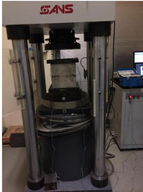
FIG. 3. Test setup consisting of compression machine, strain gauges and data logger.
