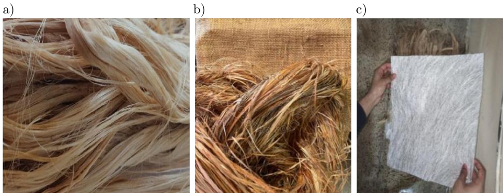
FIG. 1. Fibers used in the study: a) ramie fiber, b) hemp fiber, c) glass fiber.
