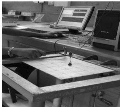
FIG. 6. Experimental setup for modal analysis.
