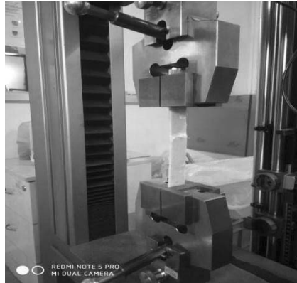
FIG. 3. Experimental setup for tensile test.
