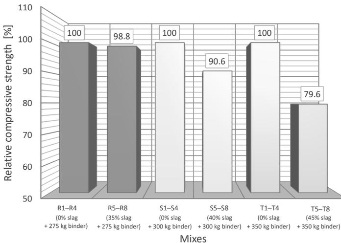
FIG. 2. Relative compressive strength at 28 days.
