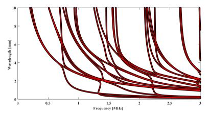
FIG. 16. Superposition of  $\lambda$ -dispersion curves: red points by GUIGUW vs. black circles by SAFE.
