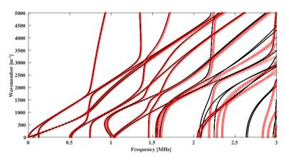
FIG. 7. Wavenumber dispersion curves by SAFE: red circles for  $N_{el} = 12$  vs. black points for  $N_{el} = 18$ .
