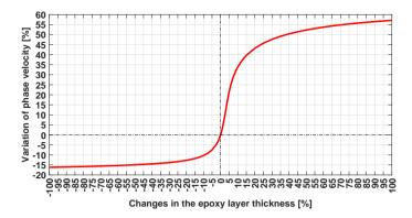
FIG. 24. The quantity  $\Delta V_P/V_P$  in relation to the variation in the epoxy layer thickness for the S0 mode at the frequency f = 0.12 MHz.
