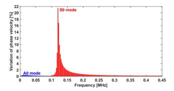
FIG. 22. The variation in the phase velocity  $\Delta V_P/V_P$  when the thickness of the epoxy layer is increased by 5% for the A0 mode and the S0 mode.
