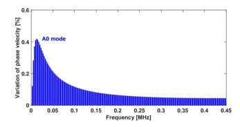
FIG. 23. Zoom at the variation in the phase velocity  $\Delta V_P/V_P$  when the thickness of the epoxy layer is increased by 5% for the A0 mode.
