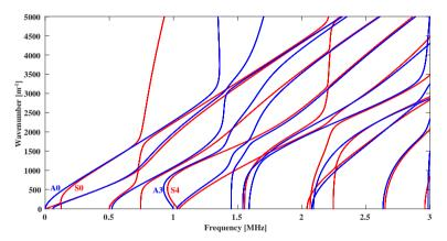
FIG. 9. Wavenumber dispersion curves of the planar tri-layer aluminum/epoxy/aluminum structure.
