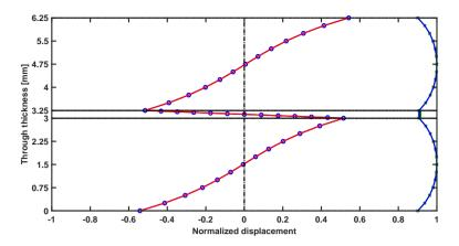
FIG. 18. Normalized displacements  $\mathbf{u}_x$  and  $\mathbf{u}_y$  at f = 200 kHz for the A0 mode: red  $(\mathbf{u}_x)$  and blue  $(\mathbf{u}_y)$  solid lines by the SAFE method vs. blue circles and green cross by the GUIGUW program.
