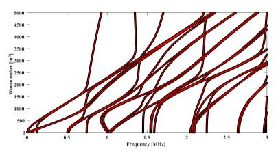
FIG. 13. Superposition of k-dispersion curves: red points by GUIGUW vs. black circles by SAFE.
