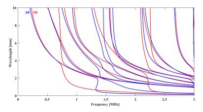
FIG. 12. Wavelength dispersion curves of the planar tri-layer aluminum/epoxy/aluminum structure.
