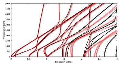
FIG. 6. Wavenumber dispersion curves by SAFE: red circles for  $N_{el} = 9$  vs. black points for  $N_{el} = 18$ .
