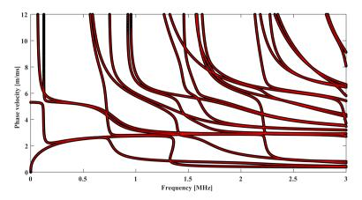
FIG. 14. Superposition of  $V_P$ -dispersion curves: red points by GUIGUW vs. black circles by SAFE.
