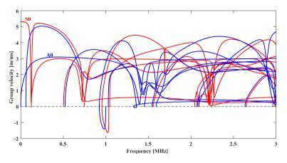
FIG. 11. Group velocity dispersion curves of the planar tri-layer aluminum/epoxy/aluminum structure.
