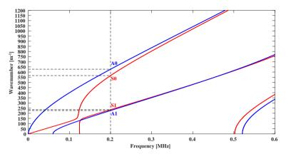
FIG. 17. Appearing Lamb modes at the frequency of 200 kHz.
