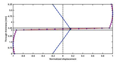
FIG. 20. Normalized displacements  $\mathbf{u}_x$  and  $\mathbf{u}_y$  at f = 200 kHz for the A1 mode: red ( $\mathbf{u}_x$ ) and blue ( $\mathbf{u}_y$ ) solid lines by the SAFE method vs. blue circles and green cross by the GUIGUW program.
