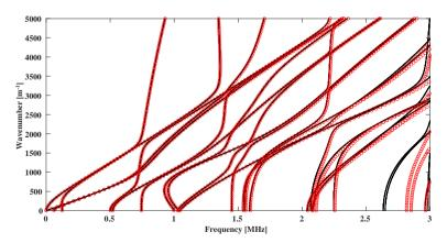
FIG. 8. Wavenumber dispersion curves by SAFE: red circles for  $N_{el} = 15$  vs. black points for  $N_{el} = 18$ .
