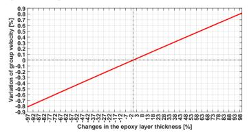
FIG. 26. The quantity  $\Delta V_G/V_G$  in relation to the variation in the epoxy layer thickness for the S0 mode at the frequency  $f = 10^{-3}$  MHz.
