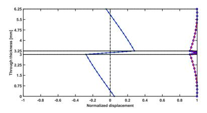
FIG. 21. Normalized displacements  $\mathbf{u}_x$  and  $\mathbf{u}_y$  at f = 200 kHz for the S1 mode: red ( $\mathbf{u}_x$ ) and blue ( $\mathbf{u}_y$ ) solid lines by the SAFE method vs. blue circles and green cross by the GUIGUW program.
