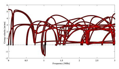
FIG. 15. Superposition of  $V_G$ -dispersion curves: red points by GUIGUW vs. black circles by SAFE.
