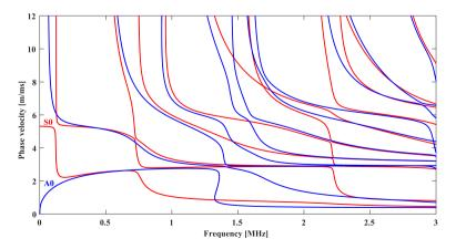
FIG. 10. Phase velocity dispersion curves of the planar tri-layer aluminum/epoxy/aluminum structure.
