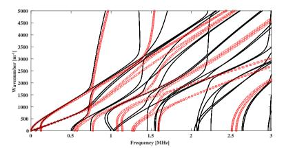
FIG. 4. Wavenumber dispersion curves by SAFE: red circles for  $N_{el} = 3$  vs. black points for  $N_{el} = 18$ .
