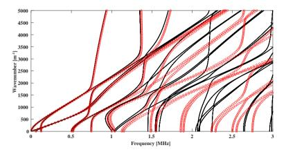
FIG. 5. Wavenumber dispersion curves by SAFE: red circles for  $N_{el} = 6$  vs. black points for  $N_{el} = 18$ .
