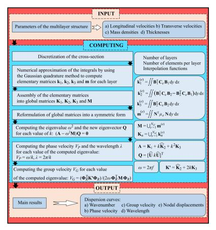
FIG. 3. Framework for calculating the dispersion curves and nodal displacements using SAFE.
