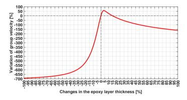
FIG. 25. The quantity  $\Delta V_G/V_G$  in relation to the variation in the epoxy layer thickness for the S0 mode at the frequency f = 0.12 MHz.
