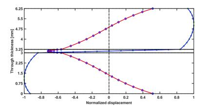
FIG. 19. Normalized displacements  $\mathbf{u}_x$  and  $\mathbf{u}_y$  at f = 200 kHz for the S0 mode: red  $(\mathbf{u}_x)$  and blue  $(\mathbf{u}_y)$  solid lines by the SAFE method vs. blue circles and green cross by the GUIGUW program.
