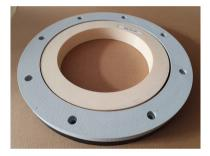
FIG. 2. 3D-printed rings of wire raceway bearing prototype.
