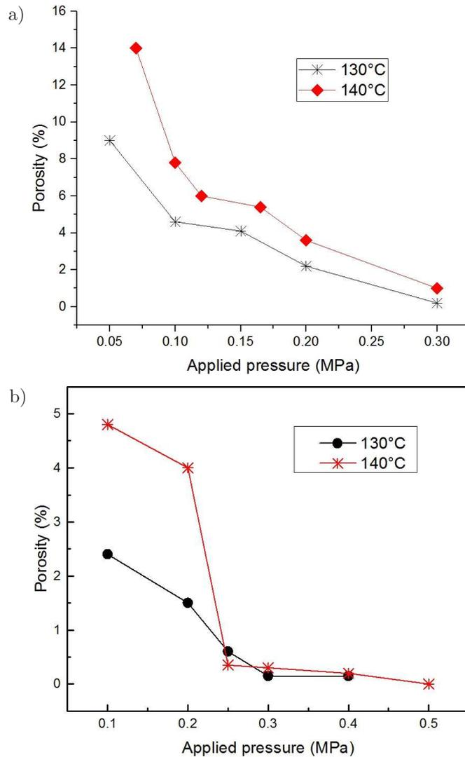
FIG. 2. Effect of curing temperature on void formation (reprinted with permission from [30]): a) epoxy BA9916 pre-preg, b) epoxy QY8911 pre-preg.
