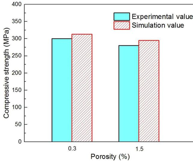
FIG. 4. Effect of void content on compressive stress (reprinted with permission from [47]).
