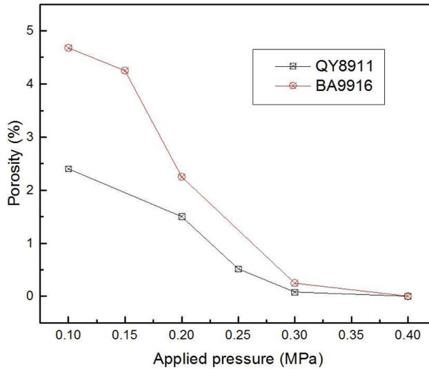
FIG. 3. Effect of resin system on void formation (reprinted with permission from [30]).
