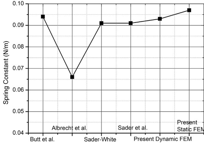
FIG. 9. Comparison of the stiffness of the V-shaped beam obtained by different methods.
