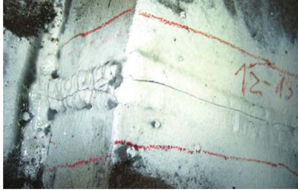
FIG. 4. Cracks weld of the crane beam stringer type "G" detected by the magnetic-powder method.
