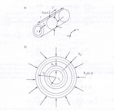
FIG. 1. Dynamic model of the three-layer shell with damping for the axially symmetric non-uniform loading.
