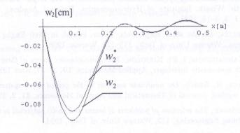
FIG. 3. The trajectory of dynamical displacements of a movable point of the viscoelastic three-layer cylindrical shell with the velocity and the various times for the moving force:a) for the Kirchhoff's-Love model, b) for the Mindlin model.
