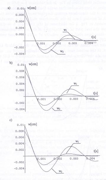
FIG. 2. Free vibrations of the three-layer system of two cylindrical shells coupled by a viscoelastic interlayer for  $X_0 = 0.51$  and various thicknesses of the interlayers: a)  $r_1 = 0.02$  m,  $r_2 = 0.05$  m, h = 0.01 m; b)  $r_1 = 0.02$  m,  $r_2 = 0.06$  m, h = 0.02 m; c)  $r_1 = 0.02$  m,  $r_2 = 0.07$  m, h = 0.03 m.
