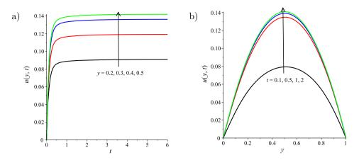
FIG. 3. Velocity profile across the channel: a) with increasing y, b) with increasing time t.
