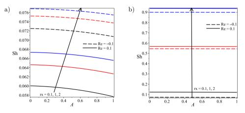
FIG. 20. Sherwood number Sh vs. pressure gradient A with increasing rx and Re: a) at y = 0, b) at y = 1.
