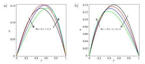
FIG. 6. Steady-state velocity profiles with increasing Re: a) Re > 0, b) Re < 0.
