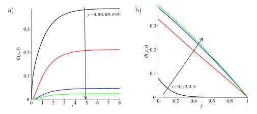
FIG. 4. Temperature profile across the channel: a) with increasing y, b) with increasing time t.
