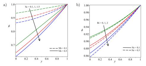
FIG. 11. Steady-state concentration profiles with increasing Sc, Nb (a) and Bi, Nr (b).
