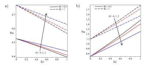
FIG. 17. Nusselt number Nu vs. Eckert number Ec with increasing M and Bi: a) at y = 0, b) at y = 1.
