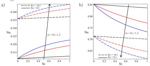
FIG. 18. Nusselt number Nu vs. Schmidt number Sc with increasing rx and Ec: a) at y = 0, b) at y = 1.
