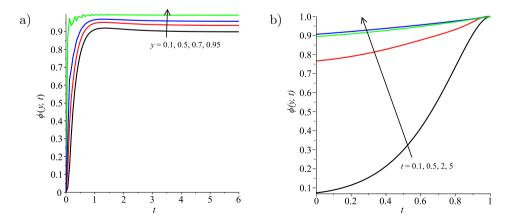
FIG. 5. Concentration profile across the channel: a) with increasing y, b) with increasing time t.
