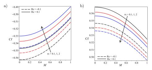
FIG. 15. Skin friction Cf vs. magnetic field parameter M with increasing rx and Re: a) at y = 0, b) at y = 1.
