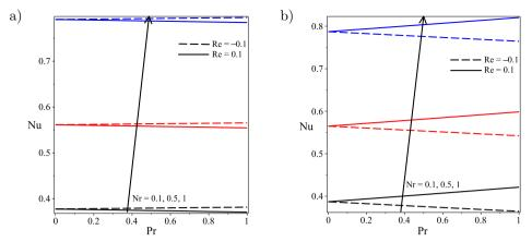
FIG. 19. Nusselt number Nu vs. Prandtl number Pr with increasing Nr and Re: a) at y = 0, b) at y = 1.
