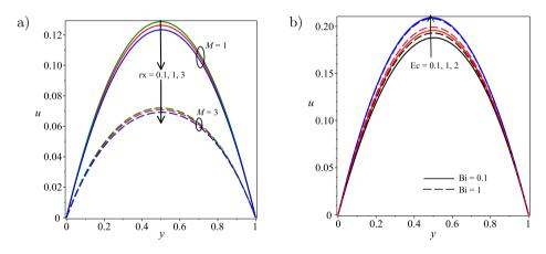
FIG. 8. Steady-state velocity profiles with increasing rx, M (a) and Ec, Bi (b).
