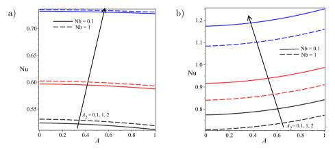
FIG. 16. Nusselt number Nu vs. pressure gradient A with increasing  $A_2$  and Nb: a) at y = 0, b) at y = 1.
