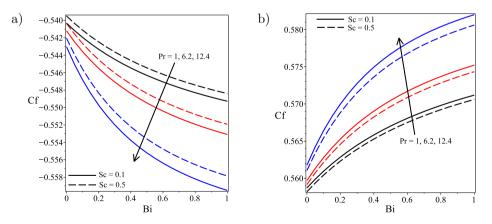
FIG. 13. Skin friction Cf vs. Biot number Bi with increasing Pr and Sc: a) at y = 0, b) at y = 1.
