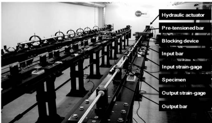
FIG. 3. Dynamic direct tensile testing set-up.
