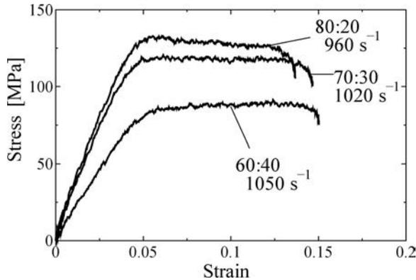
FIG. 5. Effect of PBAT content on stress-strain curves at strain rates of 960–1050 s<sup>-1</sup>.
