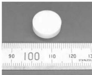
FIG. 2. Photograph of a dynamic compressive test specimen.
