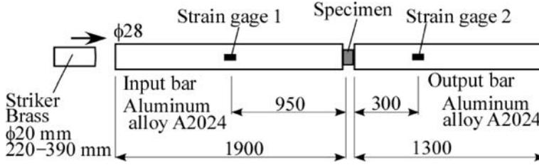
FIG. 3. Experimental setup for split Hopkinson pressure bar method (Kolsky bar).
