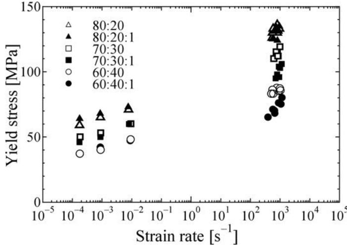
FIG. 8. Effect of strain rate on maximum stress.
