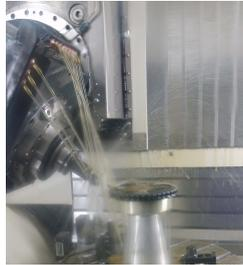
FIG. 10. End milling process of cycloidal gears.
