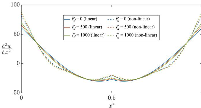
**FIG. 3.** Curvatures corresponding to the non-linear deflection response function for various excitation levels.
