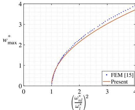
FIG. 2. Comparison of the frequency ratios of a beam resting on translational spring near the second mode.
