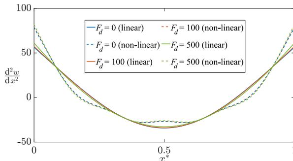
**FIG. 7.** Curvatures corresponding to the non-linear deflection response function for various excitation levels.
