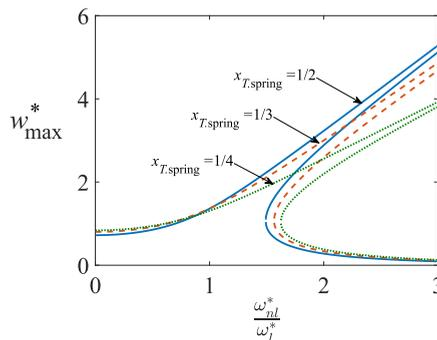
FIG. 6. The response curves based on the multimode approach of a clamped-clamped beam resting on translational spring for various spring positions.
