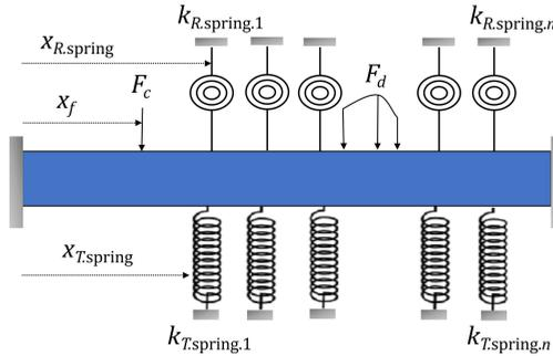
FIG. 1. Physical model of an Euler-Bernoulli beam resting on elastic point supports.
