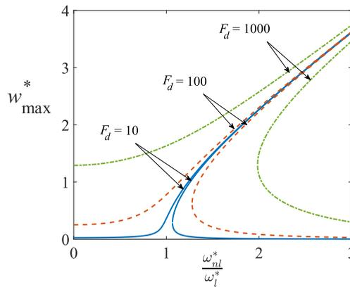
FIG. 9. The response curves based on the multimode approach of a clamped-clamped beam resting on rotational spring for various excitation levels.
