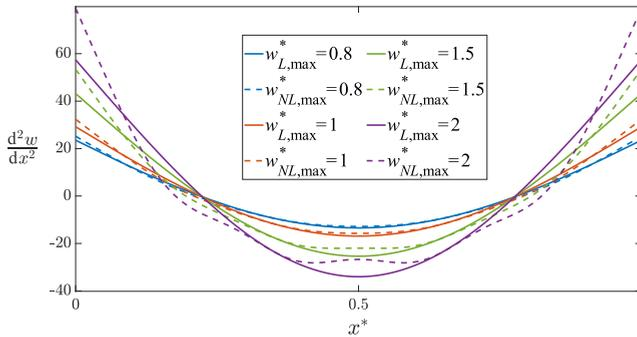
FIG. 8. Curvatures corresponding to the non-linear deflection response function for various amplitudes.
