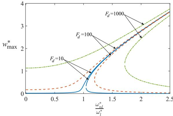
FIG. 5. The response curves based on the multimode approach of a clamped-clamped beam resting on translational spring for various excitation levels.
