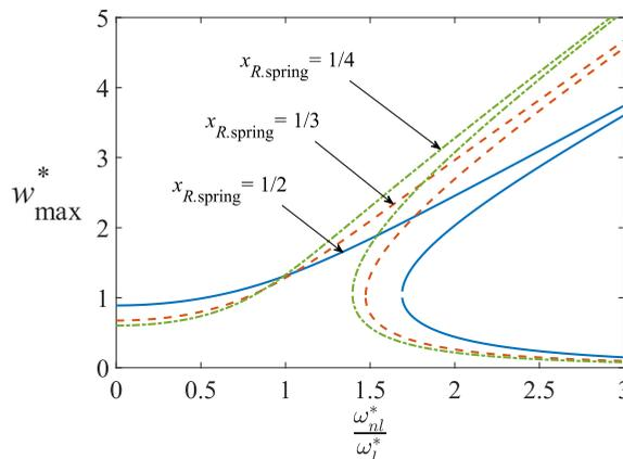
FIG. 10. The response curves based on the multimode approach of a clamped-clamped beam resting on rotational spring for various spring positions.
