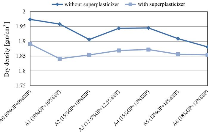
FIG. 3. Effects of glass and steel slag powders on the dry density of mortar at 28 days.
