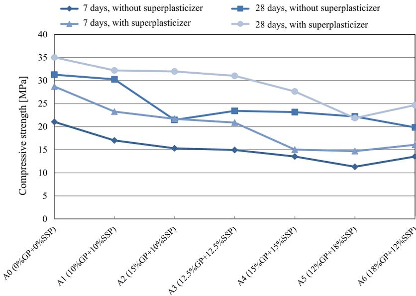
FIG. 1. Effects of glass and steel slag powders on the compressive strength of mortar.
