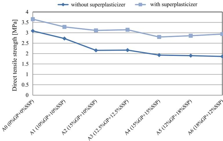
FIG. 2. Effects of glass and steel slag powders on the direct tensile strength of mortar at 28 days.
