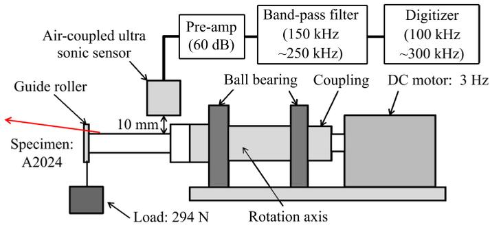
FIG. 12. Experimental setup for monitoring the AE signals during the rotary bending fatigue test.
