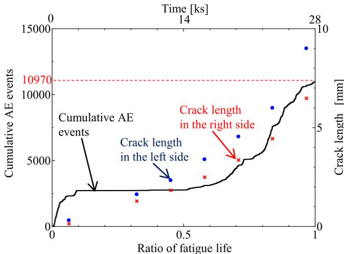
FIG. 3. Change in cumulative AE events during the plane bending fatigue test and crack observations.
