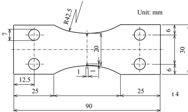
FIG. 2. Configuration of the specimen for the plane bending fatigue test.
