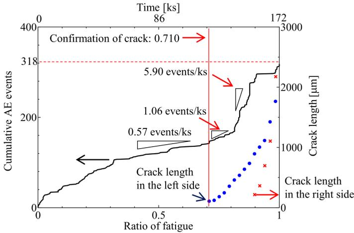
FIG. 13. Cumulative AE events and crack lengths in both sides of the specimen.
