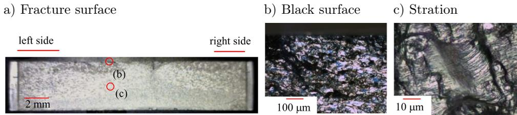
FIG. 8. Fracture surface after the plane bending fatigue test with a crack length at 0.580 of the fatigue life ratio.
