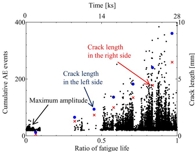
FIG. 4. Changes in the maximum amplitude during the plane bending fatigue test and crack observations.
