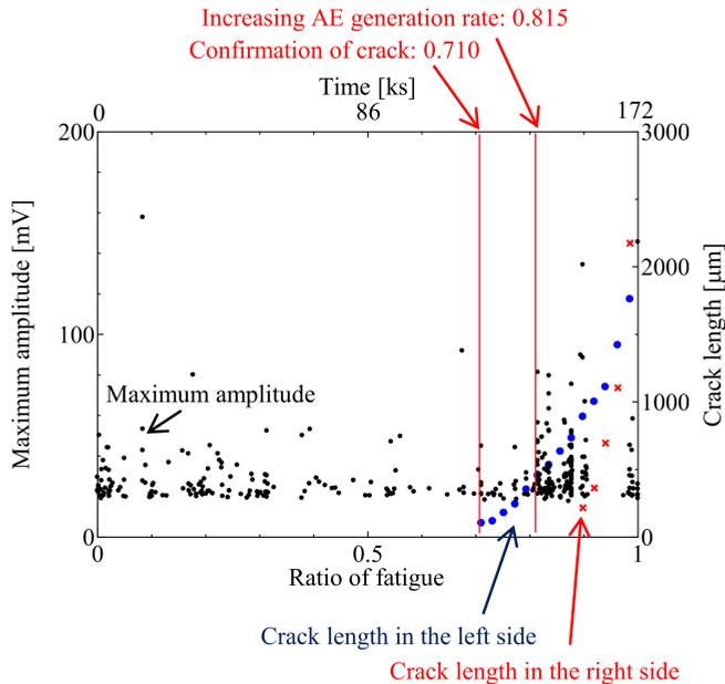
FIG. 15. Change in the maximum amplitude during the rotary bending fatigue test using the flat surface specimen, and the crack observations.
