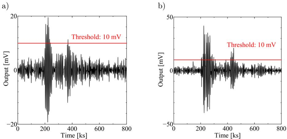
FIG. 14. AE waveforms detected at (a) 0.049 and (b) 0.815 of the fatigue life ratio.
