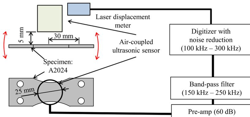
FIG. 1. Experimental setup for monitoring the AE signals during the plane bending fatigue test.
