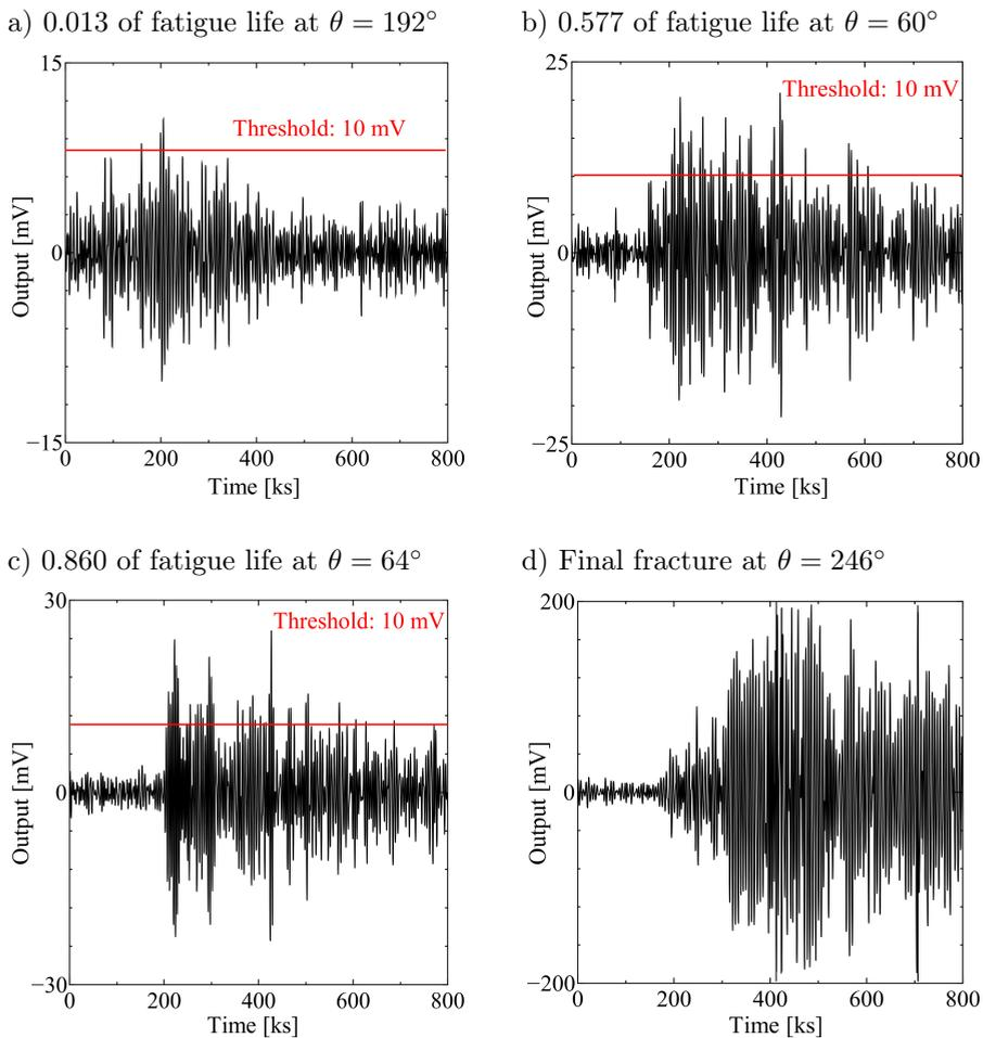
FIG. 7. AE waveforms detected at (a) 0.013, (b) 0.557, and (c) 0.860 of the fatigue life ratio and (d) the final fracture.
