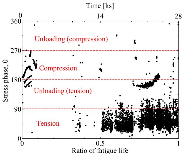
FIG. 6. Relationship between the stress phase and AE generation timing.
