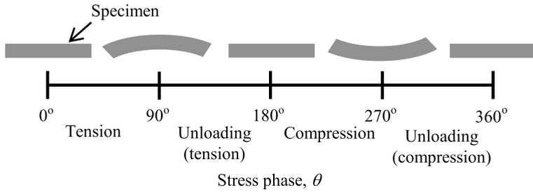
FIG. 5. Relationship between the stress phase and state of the specimen.
