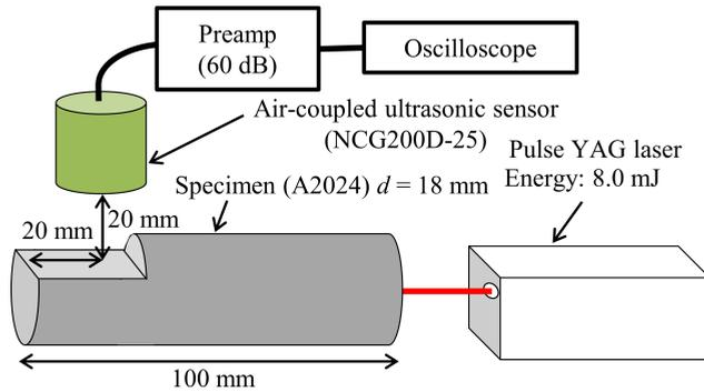
FIG. 9. Experimental setup for comparing the sensitivity of the air-coupled ultrasonic sensor on top of arc and flat surfaces.
