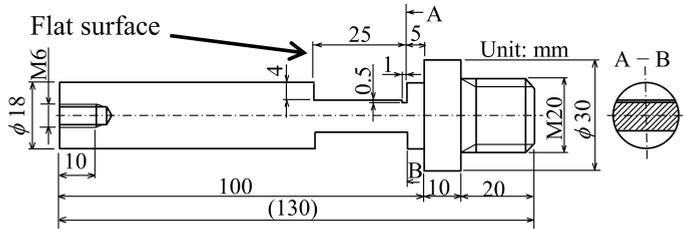
FIG. 11. Configuration of the specimen for the rotary bending fatigue test.
