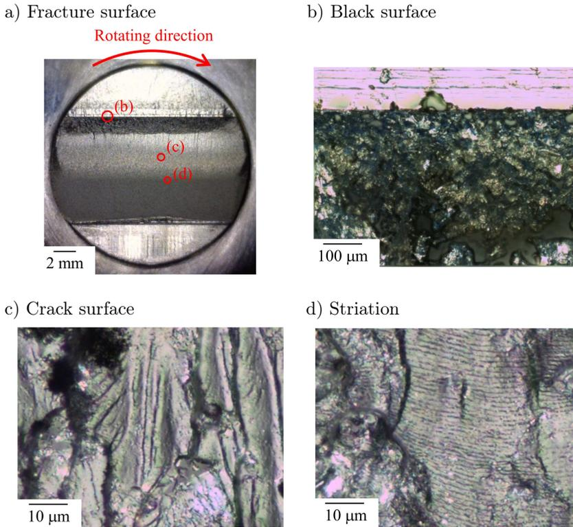
FIG. 16. Fracture surface after the rotary bending fatigue test using the specimen with a flat surface.
