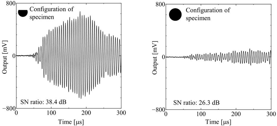
FIG. 10. Waveforms detected by the air-coupled ultrasonic sensor for the arc (right) and flat (left) surface specimens.
