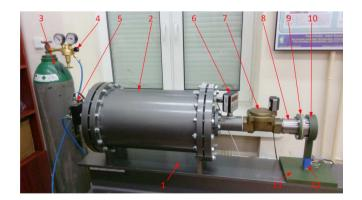
FIG. 15. Measuring stand for testing fabrics loaded with a gas pressure impulse: 1 – stand basis, 2 – pressure tank, 3 – gas cylinder (argon), 4 – pressure reducer, 5 – filling proportional valve, 6 – gauge control, 7 – valve, 8 – nozzle, 9 – sample, 10 – sample clamp, 11 – handle base, 12 – force measurement system.
