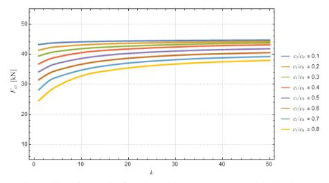
FIG. 4. The influence of  $c_1/c_0$  ratio and k parameter on critical loads values.
