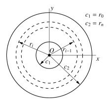
Fig. 5. Layered hollow circular cross-section.
