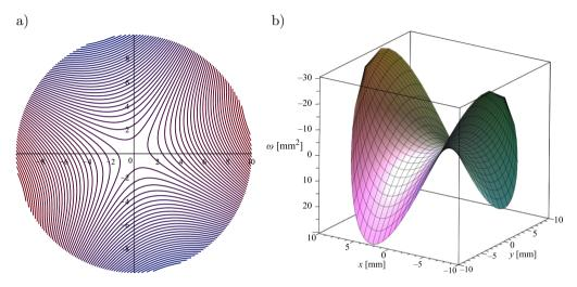
Fig. 2. Illustrations of the torsion function: a) contour lines, b) graph of the torsion function.
