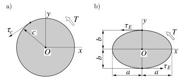
Fig. 6. Orthotropic circular (a) and isotropic elliptical (b) solid cross-sections.
