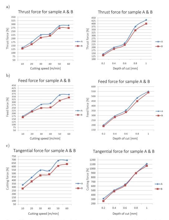
FIG. 4. Effect of cutting speed and depth of cut on the cutting forces for sample A and sample B: a) variation of thrust force of sample A and B at different cutting speeds and depth of cut, b) variation of feed force of sample A and B at different cutting speeds and depth of cut, c) variation of cutting force of sample A and B at different cutting speeds and depth of cut.
