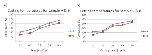
FIG. 7. Influence of feed and cutting speed on cutting temperatures of sample A (a) and sample B (b).
