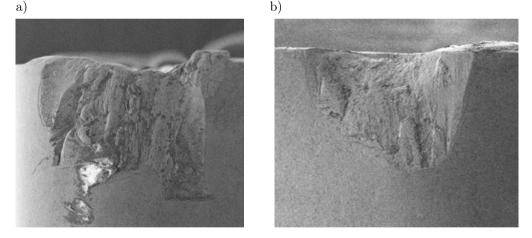
FIG. 6. Typical cutting edge wear of sample A (a) and sample B (b) at a cutting speed of 60 m/min.
