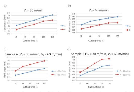
FIG. 5. Typical wear rate of sample A and sample B at cutting speeds: a) wear tests of sample A and B at  $V_c = 30 \text{ m/min}$ , b) wear tests of sample A and B at  $V_c = 60 \text{ m/min}$ , c) wear tests of sample A at  $V_c = 30$  and 60 m/min, d) wear tests of sample B at  $V_c = 30$  and 60 m/min.
