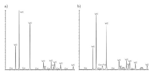
FIG. 3. X-ray spectra: a) of a WC-Co composite with 5 Wt% Co (sample A), b) of a WC-Co-Fe composite with 4.5 Wt% Co and 0.5 Wt% Fe (sample B).
