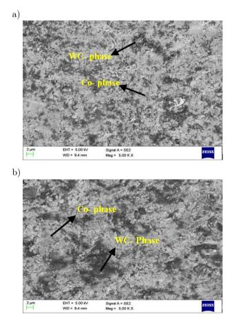
FIG. 2. SEM images of sample A (a) and sample B (b).
