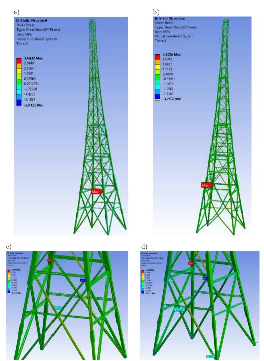
FIG. 16. Shear stress for the tower model with considered loading scenarios: a) parallel loading, b) loading at the angle  $45^{\circ}$ , with zoomed views (c), (d).
