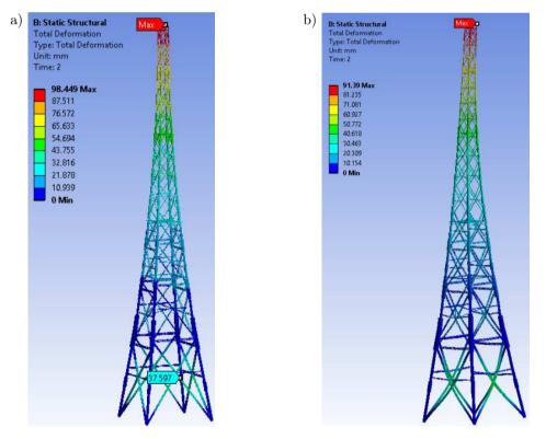
FIG. 14. Total displacement for the tower model with considered loading scenarios: a) parallel loading, b) loading at the angle  $45^{\circ}$ .
