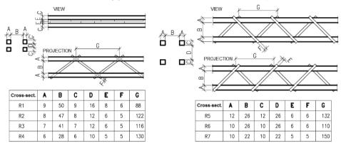
FIG. 7. Cross-sections of the four-bars purlins [2].
