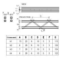
FIG. 8. Cross-sections of the four-bars diagonals [2].
