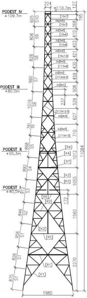
FIG. 1. General view of the tower (photo: J. Brol 2017). FIG. 2. Geometry of the tower [2].
