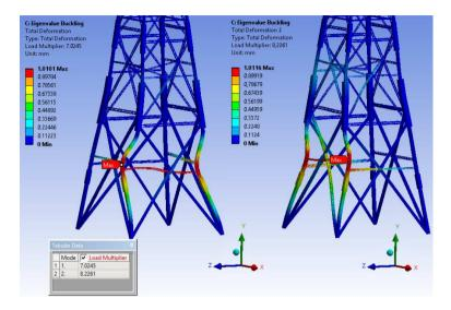
FIG. 17. First two buckling modes for the scenario of the wind acting in angle of  $45^\circ$  to the lattice.
