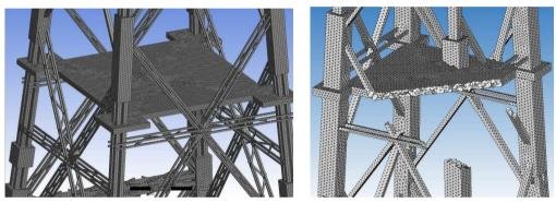
FIG. 13. View of the discretized model of tower with a cross-section.
