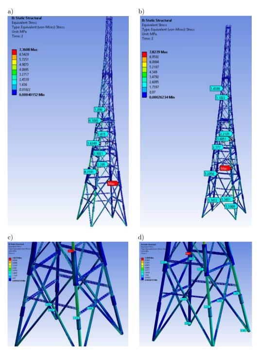
FIG. 15. Equivalent stress for the tower model with considered loading scenarios: a) parallel loading, b) loading at the angle 45°, with zoomed views (c), (d).
