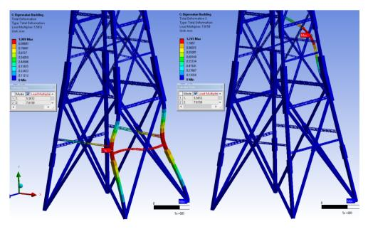
FIG. 18. First two buckling modes for the scenario of the wind acting in parallel to the lattice.
