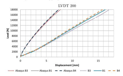
FIG. 7. The force – vertical displacement relation obtained from the numerical model and the laboratory test readout from LVDT 200.
