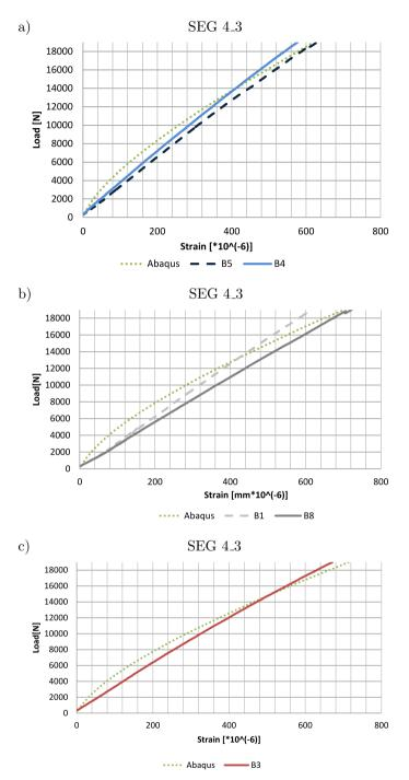
FIG. 4. The force – strain relation obtained from the numerical model and SEG 4\_3 readout for the beams: a) reinforced at the tensioned flange, b) reinforced at the compressed flange, c) bare beams.
