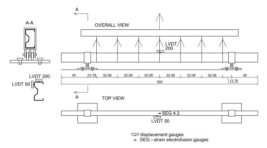
FIG. 2. Scheme of laboratory stand and layout of measuring points for displacement inductive gauges (LVDT) and strain electrofusion gauges (SEG).
