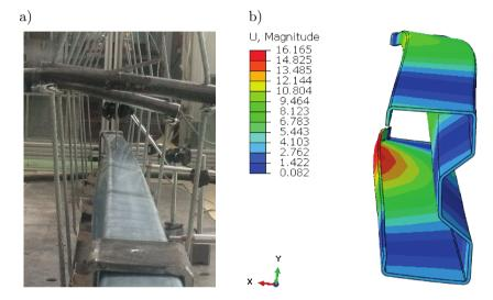
FIG. 5. Comparison of beam deformation pattern: a) laboratory test, b) numerical model (displacement map).
