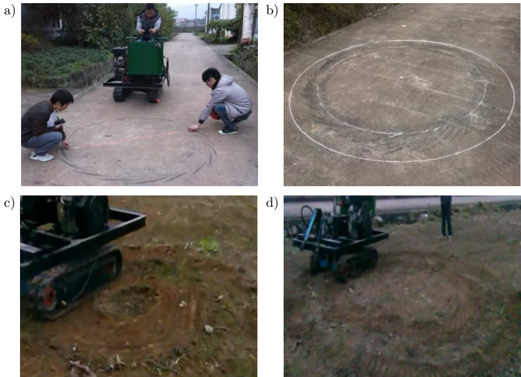
FIG. 5. The steering drive torque on different pavements: a) the unilateral steering on dry cement road, b) the free steering on dry cement road, c) the unilateral steering in the fields, d) the free steering in the fields.
