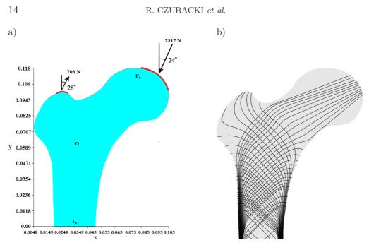
FIG. 1. a) Setting of the static problem, b) trajectories of principal stresses in the optimal body.
