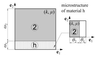
FIG. 3. The second-rank stiff laminate. The isotropic material 2 plays the role of the coating.
