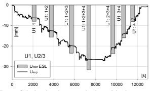
FIG. 5. Calculated and measured values of displacements in point U2/3 during different stages of test U1.
