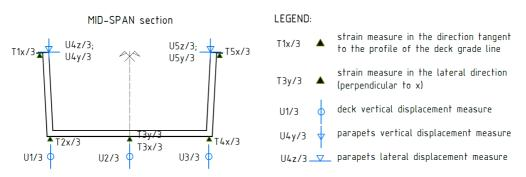
FIG. 3. Location of measurement points in mid-span section of the footbridge.
