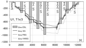
FIG. 6. Calculated and measured values of longitudinal strains in T1x/3 during different stages of test U1.
