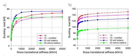
FIG. 2. The relation between buckling load and brace translational stiffness in 1D and threedimensional (3D) models ( $k_{rot} = 0 \text{ kN} \cdot \text{m/rad}$ ) for: a) torsion free, b) torsion blocked at the marginal supports.
