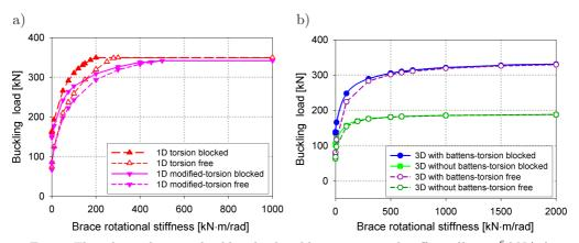
FIG. 3. The relation between buckling load and brace rotational stiffness ( $k = 10^6 \text{ kN/m}$ ) with respect to boundary conditions on the marginal supports in: a) 1D model of the truss, b) 3D model.
