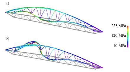
FIG. 6. Deformation at the limit state (GMNIA) for the truss with braces of stiffness: a)  $k = 10^6 \text{ kN/m}$ ,  $k_{\text{rot}} = 100 \text{ kN} \cdot \text{m/rad} - \text{imperf. I}$ ,  $k = 10^6 \text{ kN/m}$ ,  $k_{\text{rot}} = 100 \text{ kN} \cdot \text{m/rad} - \text{imperf. II}$ .
