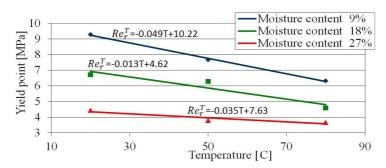
FIG. 6. Yield point vs. temperature for three moisture content levels – beech, radial direction.
