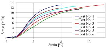
FIG. 5. The stress-strain curves for six beech specimens sheared in radial direction at  $20^{\circ}$ C and 18% moisture content.
