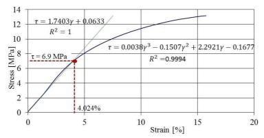
FIG. 4. The stress-strain curve for beech specimen sheared in radial direction at  $20^{\circ}$ C and 18% moisture.
