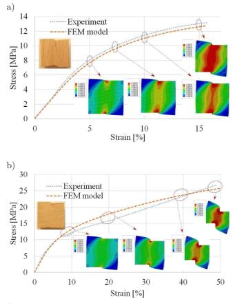
FIG. 7. a) The stress-strain curves for beech specimen sheared in radial direction at  $20^{\circ}$ C and 18% moisture, b) the stress-strain curves for beech specimen sheared in longitudinal direction at  $20^{\circ}$ C and 18% moisture.
