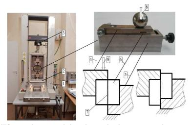
FIG. 3. MTS strength tester including climate chamber: 1 - strength tester, 2 - climate chamber, 3 - load cell (measuring the applied force), 4 - movable jaw of shear test device, 5 - fixed jaw of shear test device, 6 - specimen, 7 - surface of cutting, 8 - load of strength tester.
