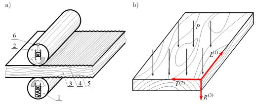
FIG. 1. a) Treatment of the surface layer of natural material by hot rolling: 1 – bottom roller, 2 – top roller, 3 – chipboard, 4, 5 – top and bottom layers of natural veneer, 6 – applied force,
