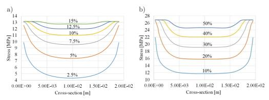
FIG. 8. a) The stress-cross-section distance curves for beech specimen sheared in radial direction, b) the stress-cross-section distance curves for beech specimen sheared in longitudinal direction.
