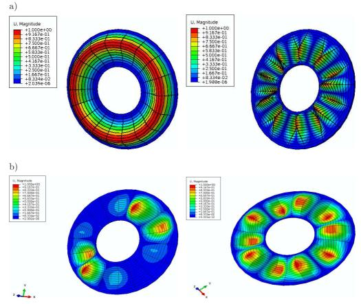
FIG. 3. Plate buckling forms for: a) non-damaged laminas, b) damaged laminas.
