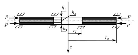
FIG. 1. Scheme of three-layered annular plate with composite facings.
