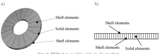
FIG. 2. FEM plate models: a) basic, b) simplistic.
