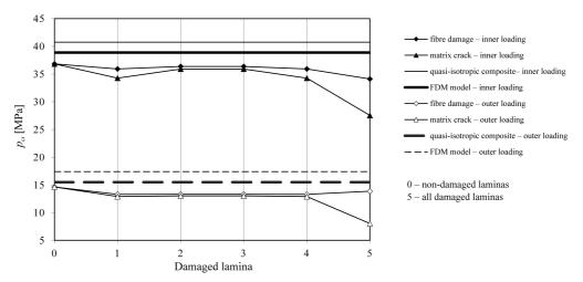
FIG. 4. Distribution of the critical static stress for plates with damaged laminas of facings.
