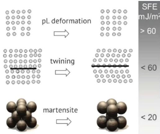
FIG. 1. Nature of microstructural changes during deformation in dependency of stacking fault energy.
