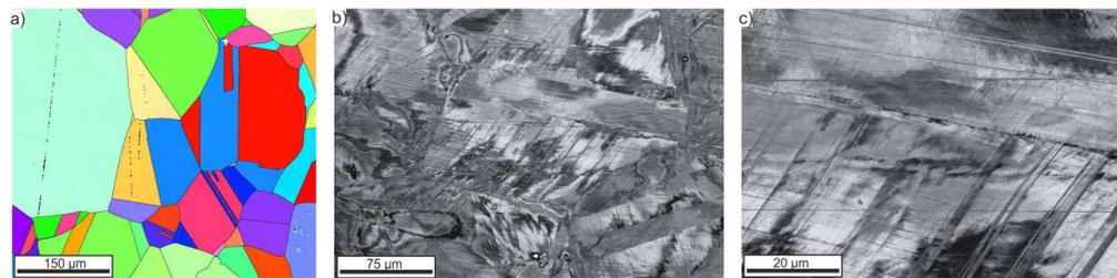
FIG. 5. SEM-micrographs, (a) EBSD mappings with grain orientation of microstructure before tensile test, (b) and (c) ECCI after 20% elongation of HSD<sup>®</sup> 600.
