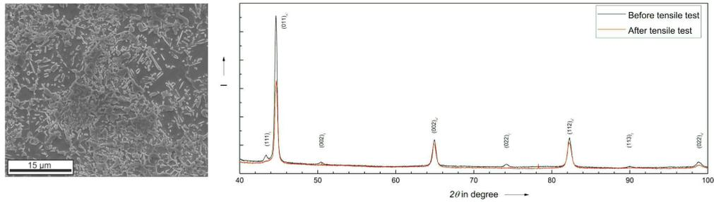
FIG. 3. SEM-micrograph of initial microstructure and diffractograms before and after tensile test of HCT 780T.
