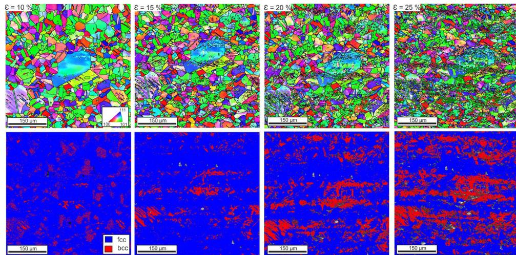
FIG. 4. EBSD mappings with grain orientation (above) and phase distribution (below) from AISI 347 at different tensile strains.
