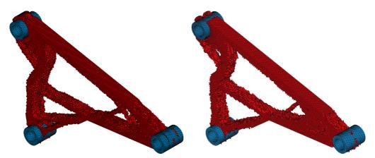
FIG. 2. Final topology for regular (left) and irregular (right) lattice.
